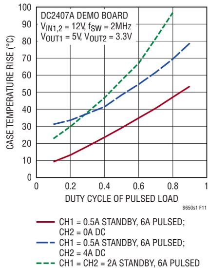
Figure 11. Case Temperature Rise vs 6A Pulsed Load
