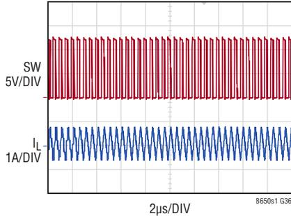
$12V_{IN}$  TO  $5V_{OUT}$  AT 100mA
