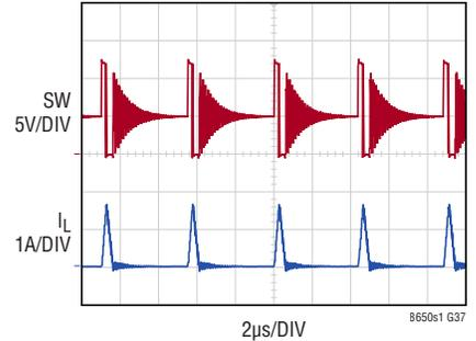
$12V_{IN}$  TO  $5V_{OUT}$  AT 100mA
