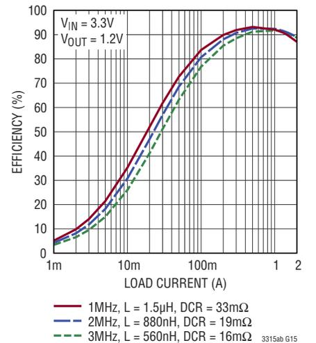
**TYPICAL PERFORMANCE CHARACTERISTICS**  $T_A = 25^\circ\text{C}$ ,  $V_{IN} = 3.3\text{V}$ , unless otherwise noted.
