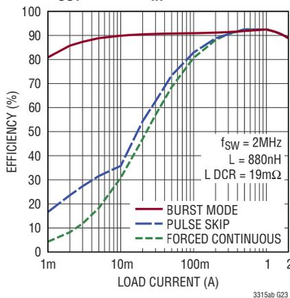
**Efficiency vs I<sub>LOAD</sub>,
