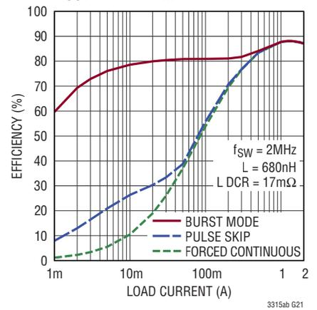
**Efficiency vs I<sub>LOAD</sub>,
