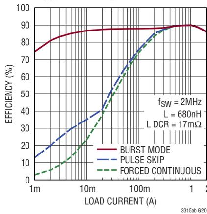
**Efficiency vs I<sub>LOAD</sub>,
