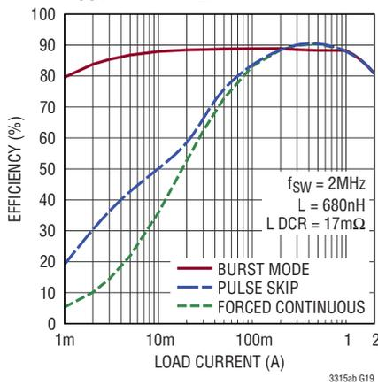
**Efficiency vs I<sub>LOAD</sub>,
