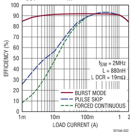
**Efficiency vs I<sub>LOAD</sub>,
