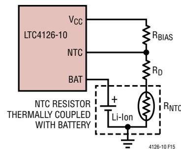
**Figure 15. NTC Thermistor Connection with Desensitizing Resistor  $R_D$**
