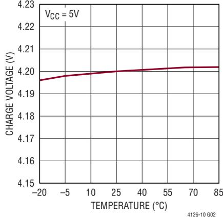
**Charge Voltage vs Temperature ( $V_{SEL} = 0V$ )**
