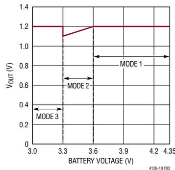
**Figure 3.  $V_{OUT}$  vs Battery Voltage at  $I_{OUT} = 0$**
