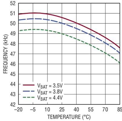
**DC/DC Switching Frequency in 2:1 Mode vs Temperature**
