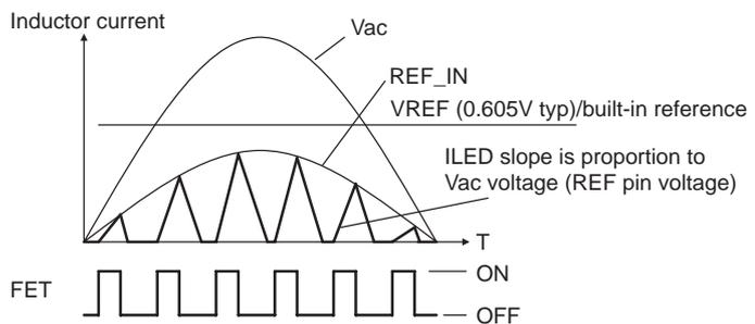
$$I_{pk} = (V_{ac} - V_f) / L \times T_c = V_f / L \times T_d$$
