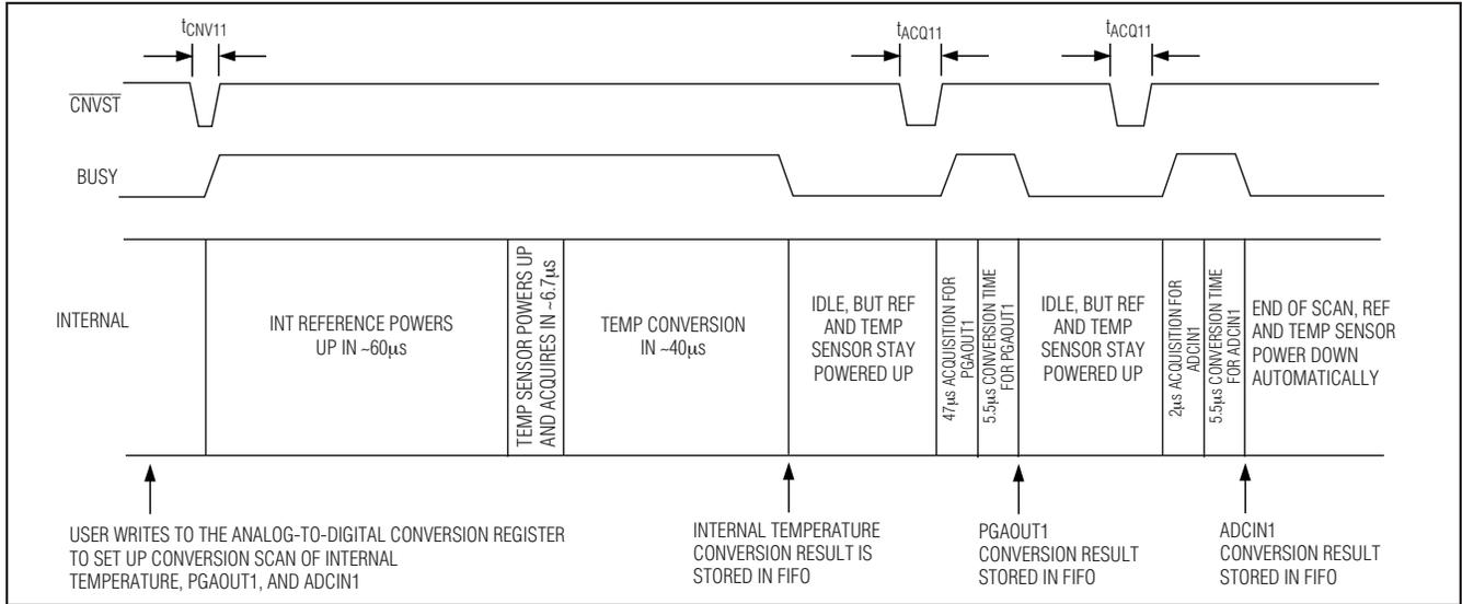
Figure 23. ADC Clock Mode 11, Example 1
