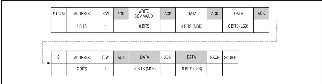
Figure 12. Write/Readback Sequence
