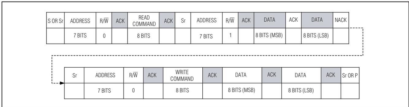
Figure 13. Read-Modify-Write Sequence
