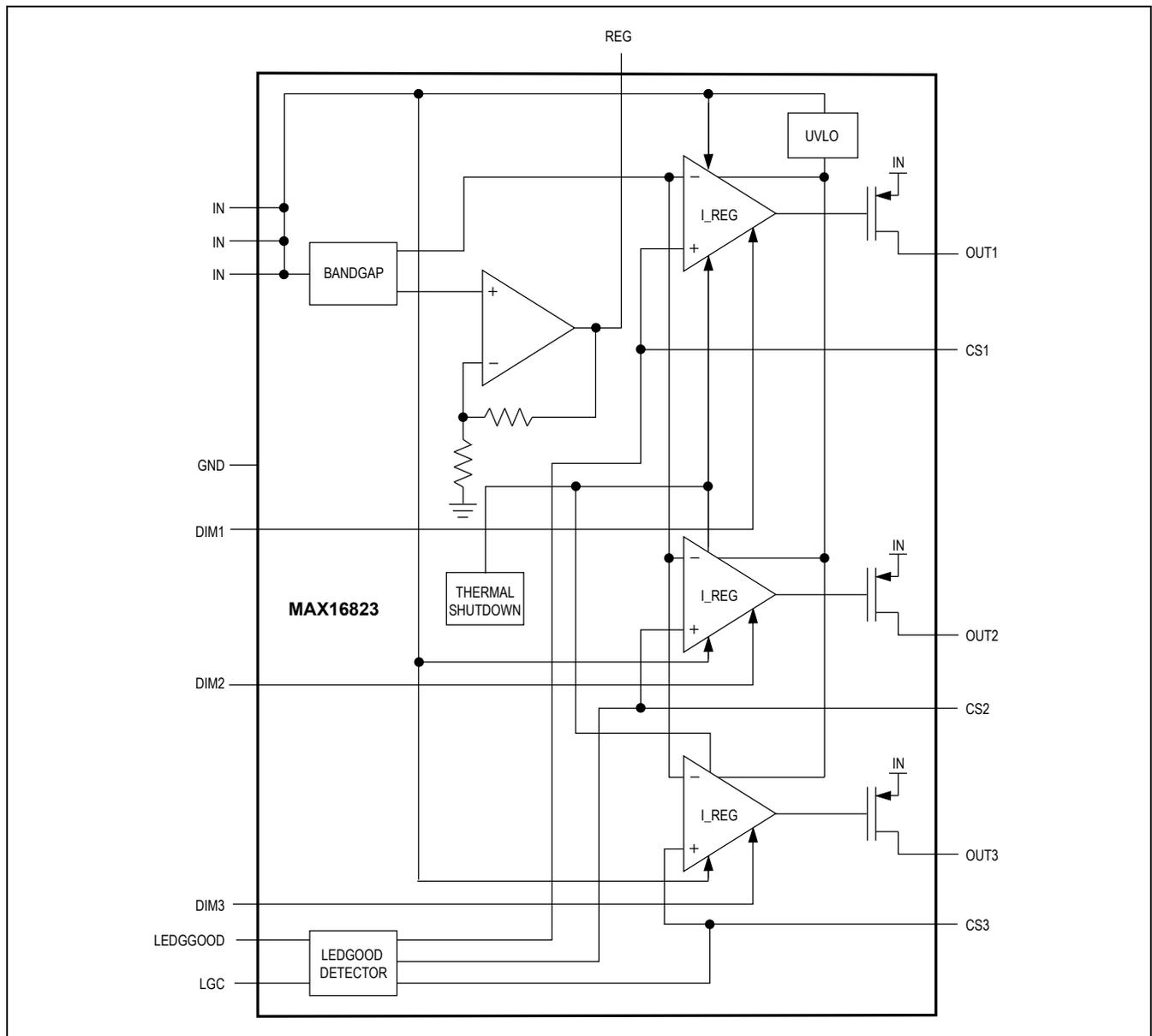
Pulse-Dimming Inputs (DIM\_)
