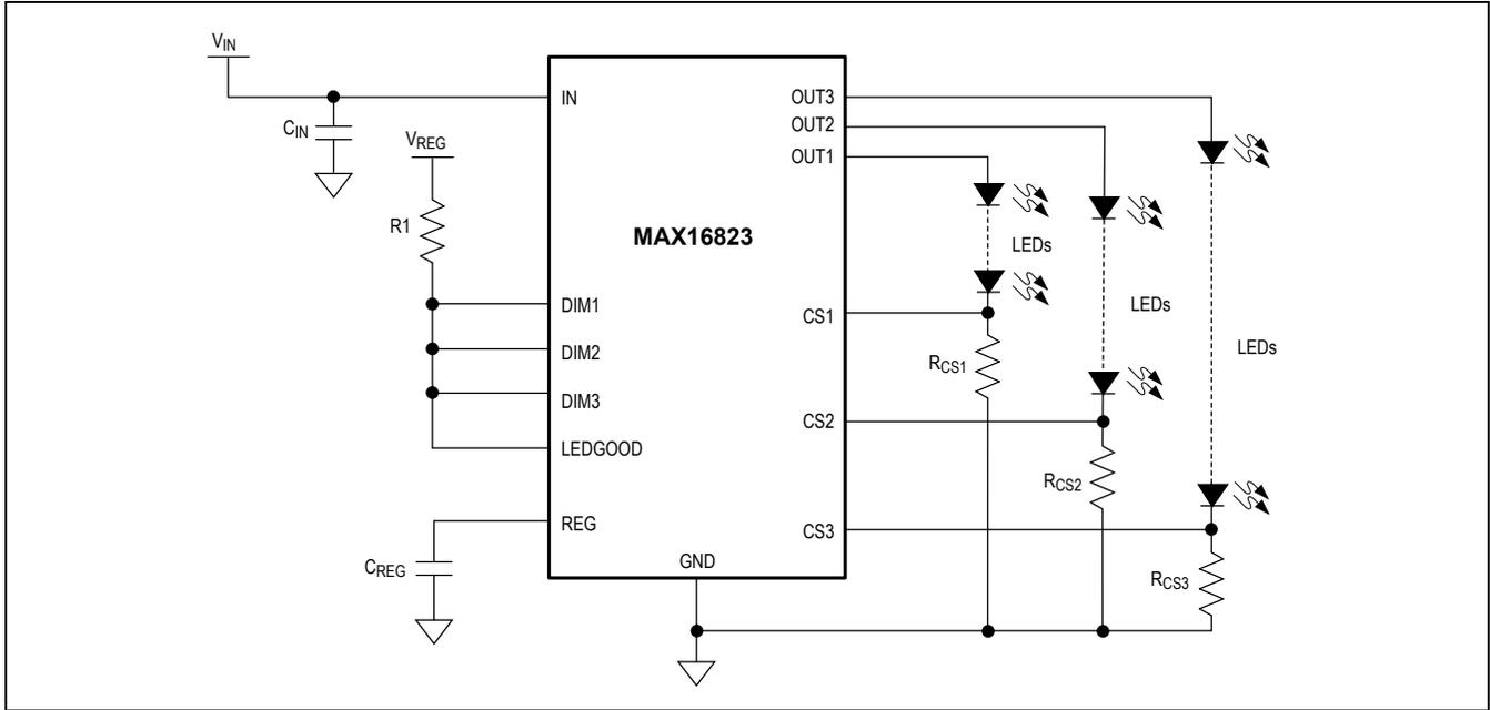
Figure 3. Output\_Latch-Off
