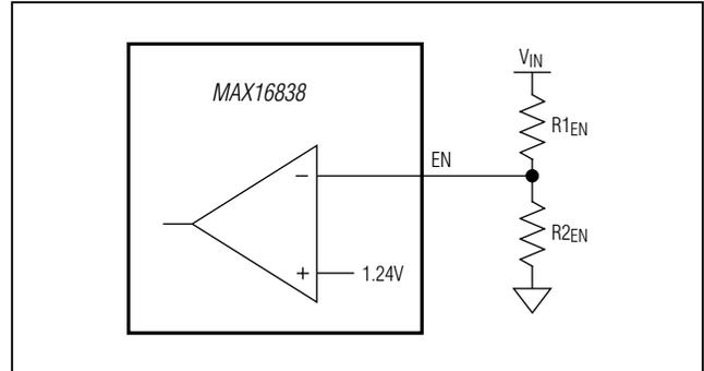
Figure 3. Setting the MAX16838 Undervoltage Lockout Threshold
