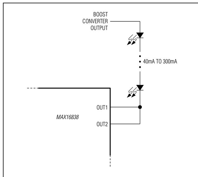
Figure 2. Configuration for Higher LED String Current
