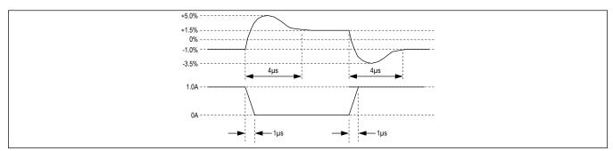
Figure 1. Load-Transient Response
