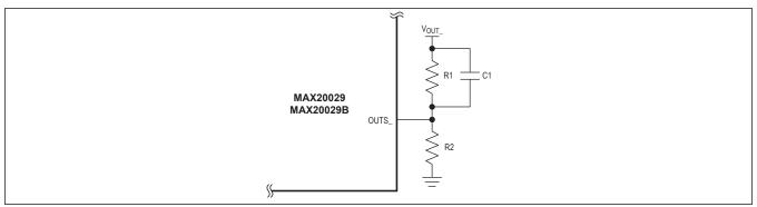
Figure 3. Adjustable Output-Voltage Configuration
