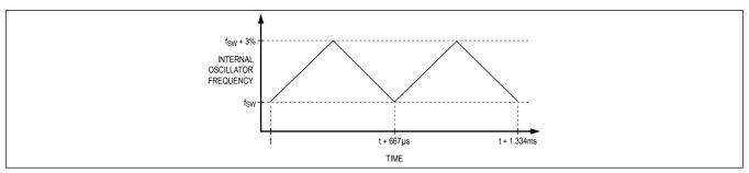
Figure 2. Effect of Spread Spectrum on Internal Oscillator
