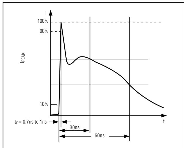
Figure 7b. IEC 1000-4-2 ESD Generator Current Waveform
