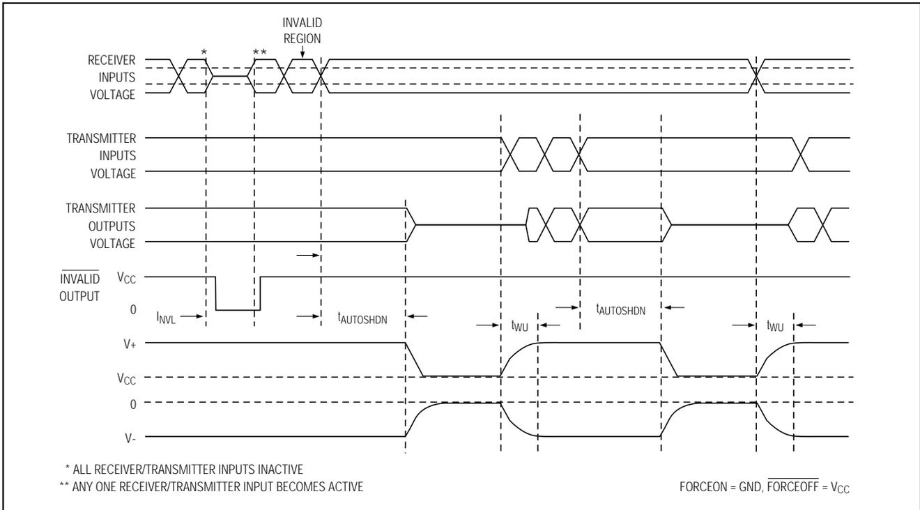
Figure 3a. AutoShutdown Plus and  $\overline{\text{INVALID}}$  Timing Diagram
