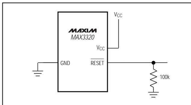
Figure 4. Ensuring  $\overline{\text{RESET}}$  Valid to  $V_{CC} = 0V$
