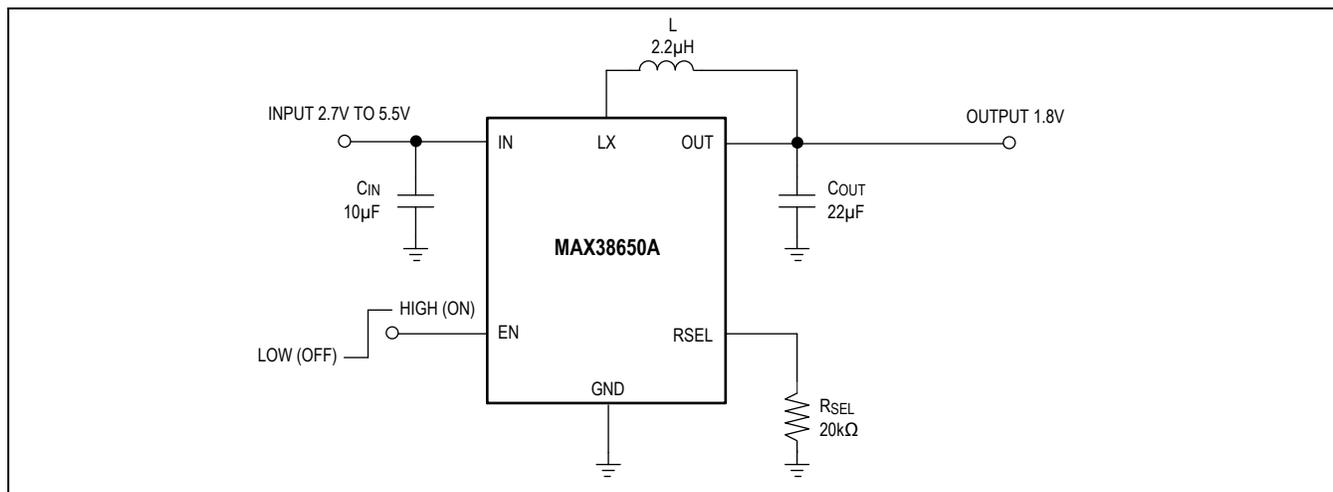
Figure 1. 1.8V Buck Converter Using the MAX38650A
