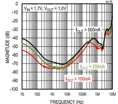
(MAX38911,  $V_{IN} = 2.1V$ ,  $V_{OUT} = 1.8V$ ,  $T_A = +25^{\circ}C$ ,  $C_{IN} = 4.7\mu F$ ,  $C_{OUT} = 4.7\mu F$ ,  $C_{BYP} = 10nF$ , unless otherwise noted.)
