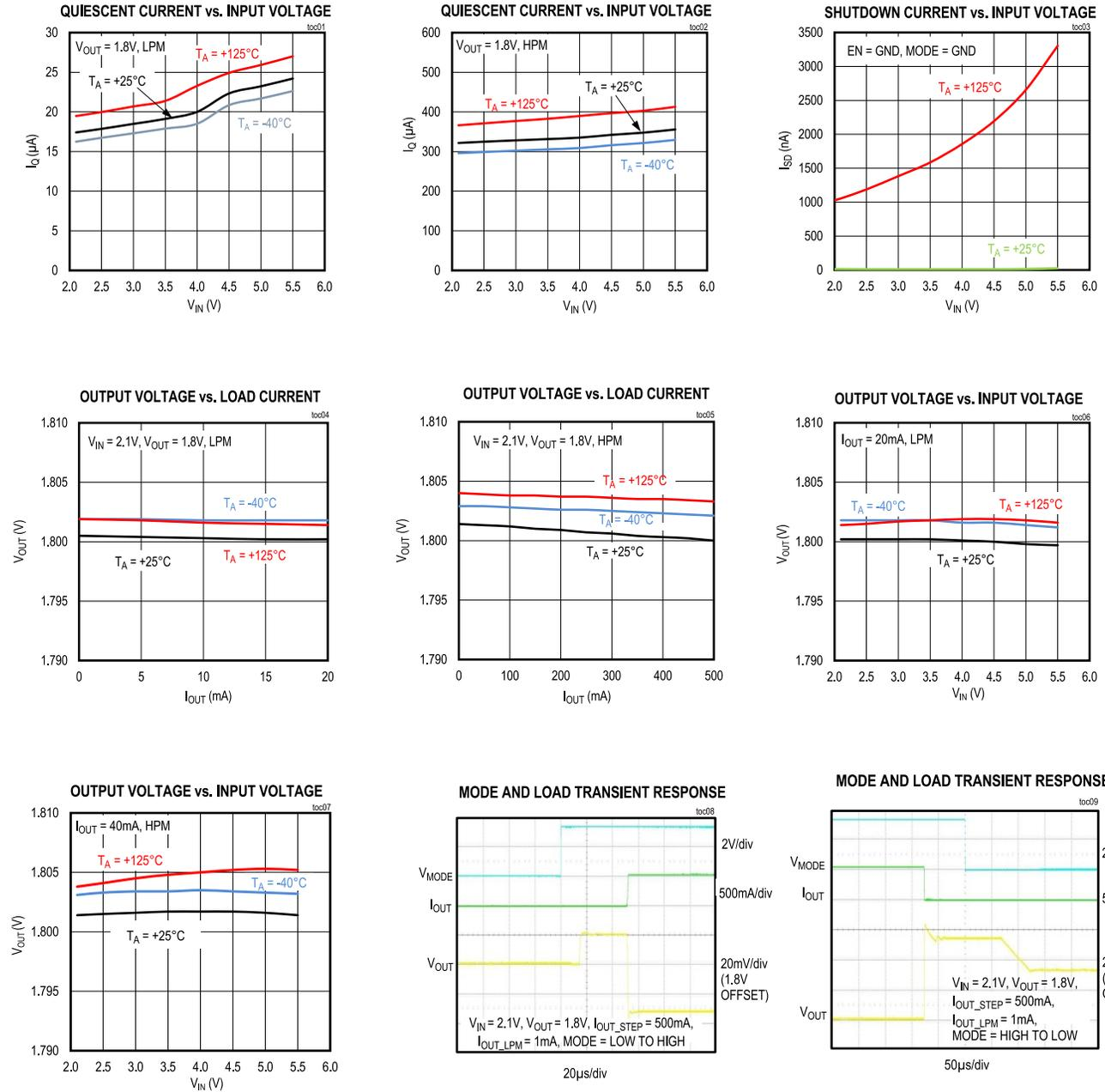
(MAX38911,  $V_{IN} = 2.1V$ ,  $V_{OUT} = 1.8V$ ,  $T_A = +25^{\circ}C$ ,  $C_{IN} = 4.7\mu F$ ,  $C_{OUT} = 4.7\mu F$ ,  $C_{BYP} = 10nF$ , unless otherwise noted.)
