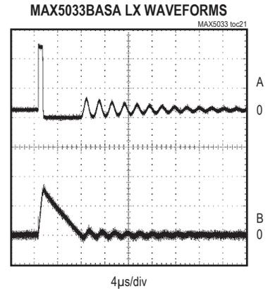
A: SWITCH VOLTAGE (LX PIN), 20V/div,  $V_{IN} = 48V$
