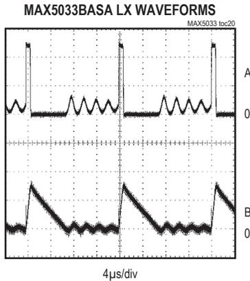
A: SWITCH VOLTAGE, 20V/div,  $V_{IN} = 48V$
