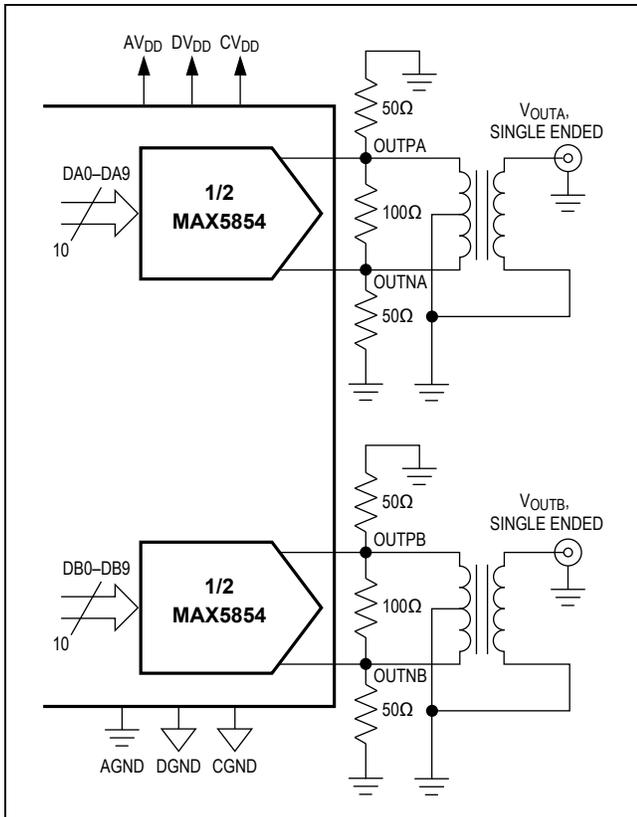
Figure 7. Application with Output Transformer Performing Differential-to-Single-Ended Conversion
