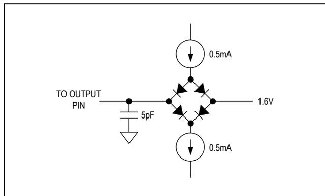
Figure 1. Load Test Circuit for CLK Outputs
