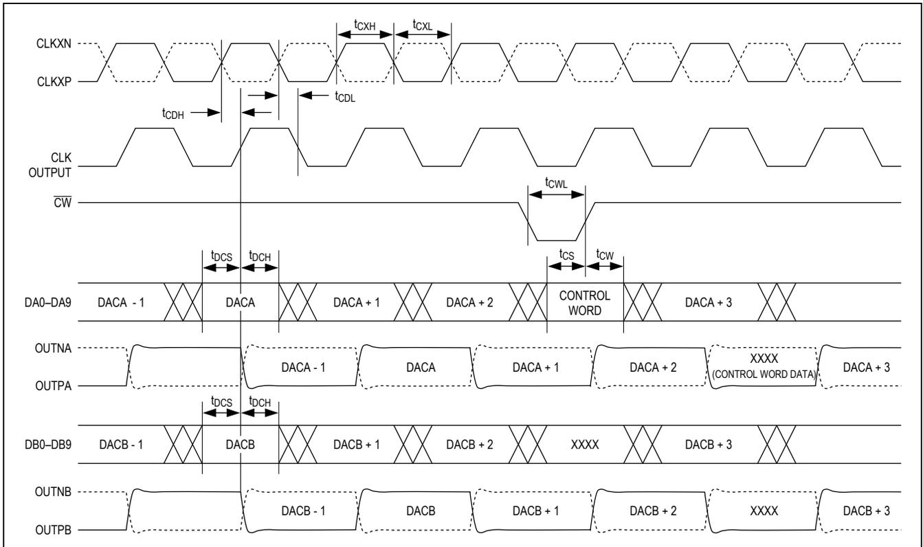
Figure 5. Timing Diagram for Noninterleaved Data Mode ( $IDE = 0$ )
