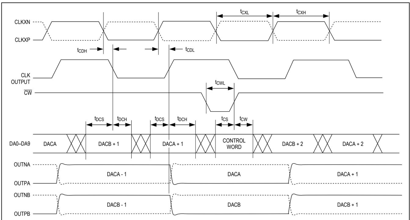
Figure 6. Timing Diagram for Interleaved Data Mode ( $IDE = 1$ )
