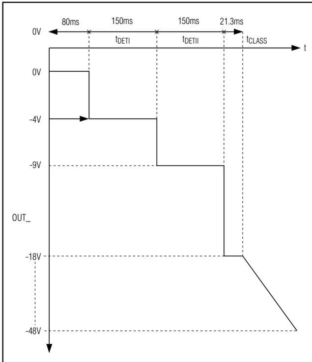
Figure 2. Detection, Classification, and Power-Up Port Sequence
