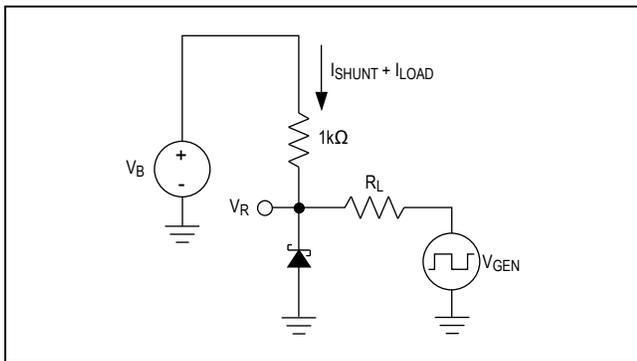
Figure 1. Load-Transient Circuit
