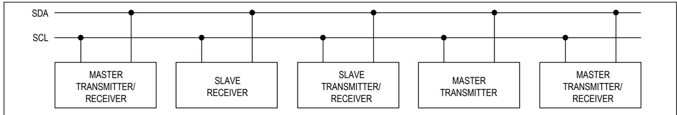
Figure 12. I<sup>2</sup>C System Configuration
