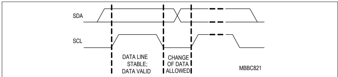
Figure 13. I<sup>2</sup>C Bit Transfer
