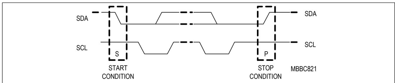
Figure 14. I<sup>2</sup>C Start and Stop
