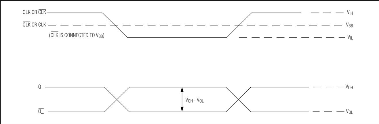
Figure 1. MAX9310A Switching Characteristics with Single-Ended Input
