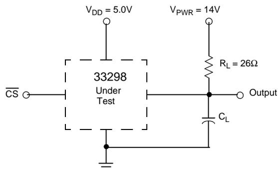
$C_L$  represents the total capacitance of the test fixture and probe.
