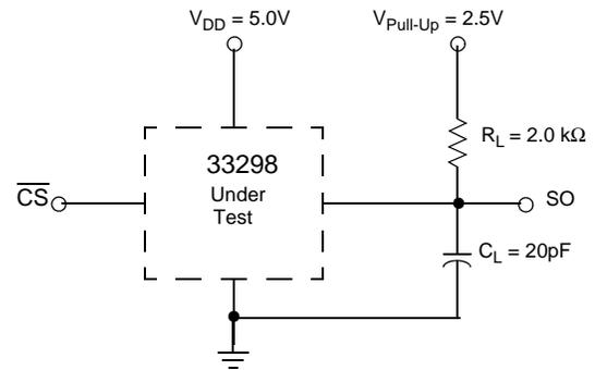
$C_L$  represents the total capacitance of the test fixture and probe.
