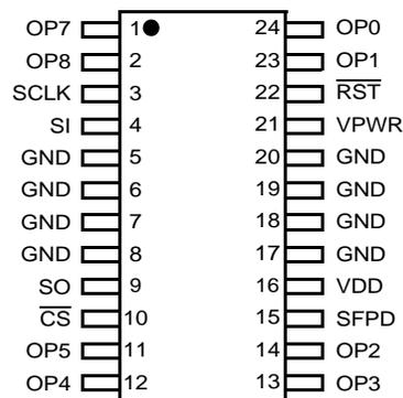
Figure 3. 33298 Pin Connections
