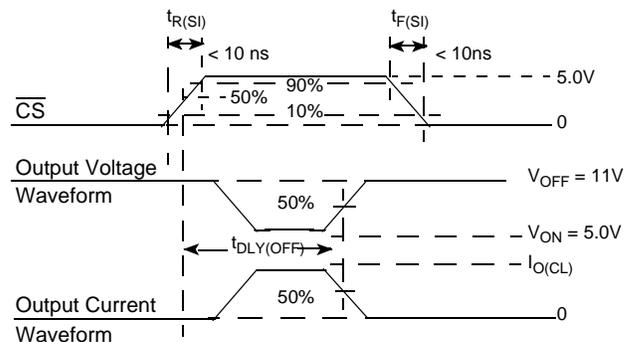
1.  $t_{PDLY(OFF)}$  is the output fault unlatch disable propagation delay time required to correctly report an output fault after CS rises. It represents an output commanded ON while having an existing output short (over-current) to supply.
