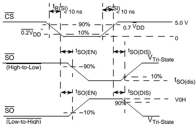
1. SO (high-to-low) waveform is for SO output with internal conditions such that SO output is low except when an output is disabled as a result of detecting a circuit fault with CS in a High Logic state, e.g. open load.
