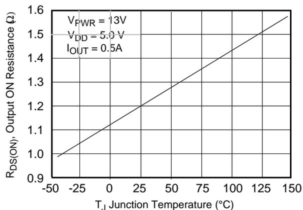
Figure 25. Maximum Output ON Resistance vs. Junction Temperature
