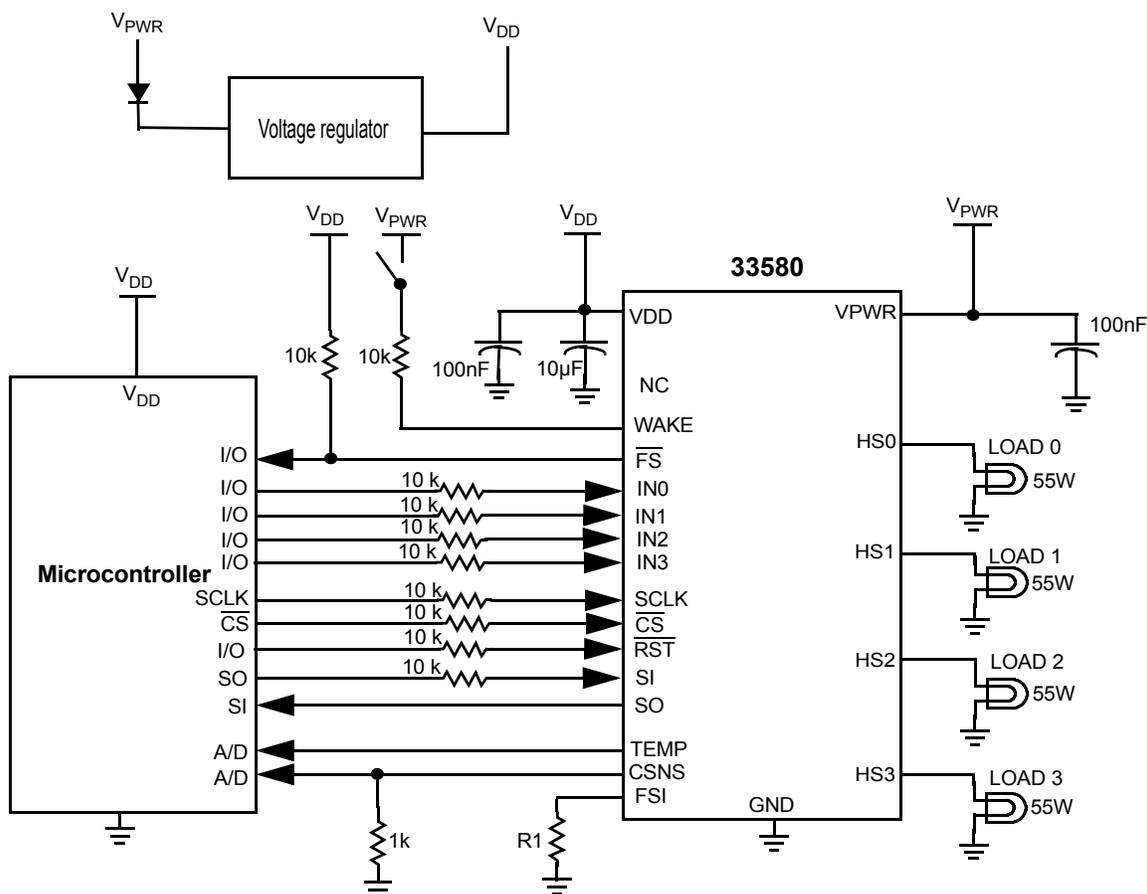
Automotive lamps do not tolerate high voltages very well. Tests of a few lamps indicate that failures can occur when 18V is applied for a few seconds. Consequently, PWM switching reduces the effective RMS voltage in order to drive bulbs safely.
