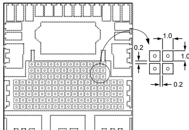
Note: Recommended via diameter is 0.5 mm. PTH (plated through hole) via must be plugged / filled with epoxy or solder mask in order to minimize void formation and to avoid any solder wicking into the via.
