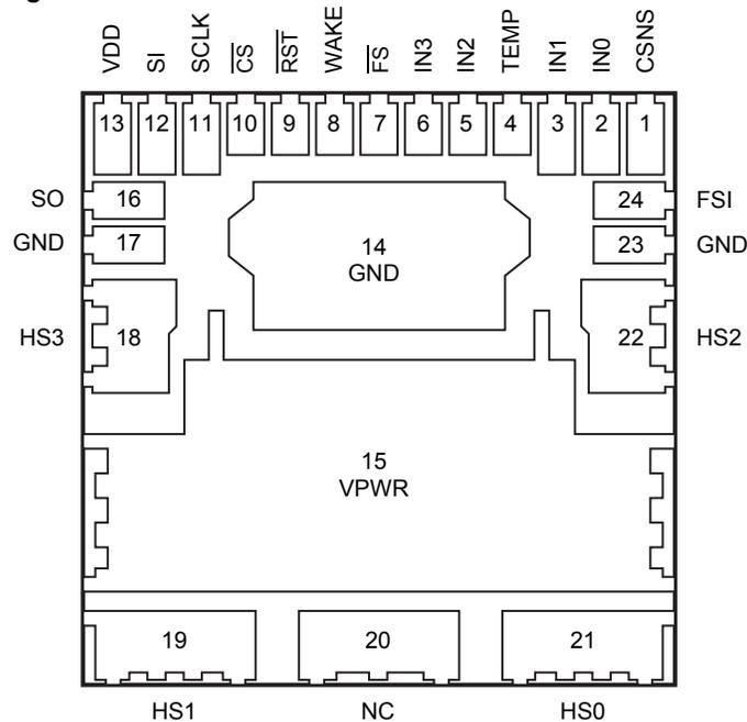
Figure 3. 33580 Pin Connections
