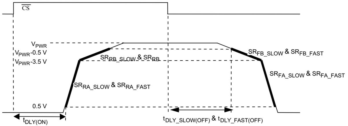
**Figure 4. Output Slew Rate and Time Delays**
