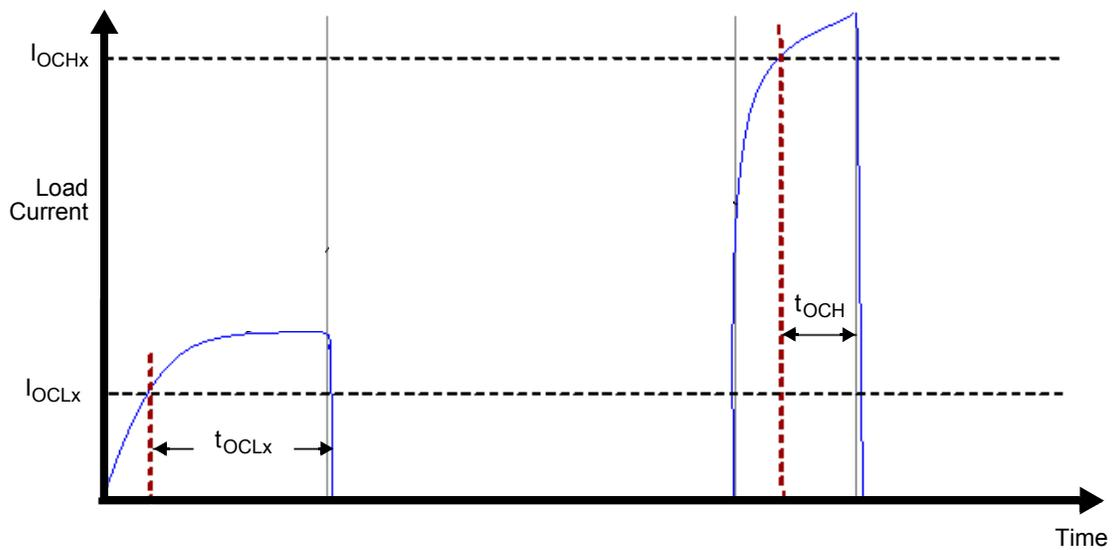
**Figure 5. Overcurrent Shutdown**
