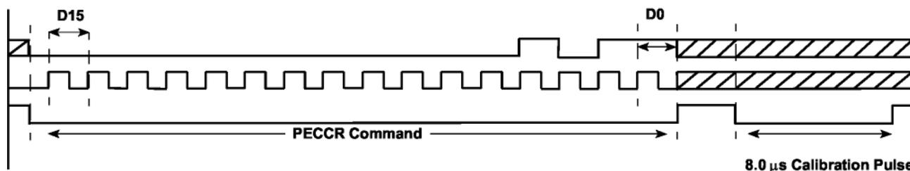
**Figure 8. Gauge Enable and Clock Calibration Example**
