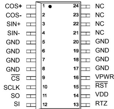
Figure 3. 33977 Pin Connections
