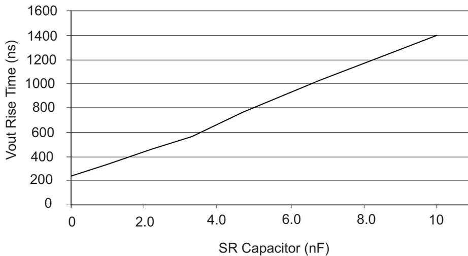
Figure 9. V<sub>OUT</sub> Rise Time vs. SR Capacitor From 10% to 90% of V<sub>OUT</sub> at 25 °C and V<sub>PWR</sub> = 13 V
