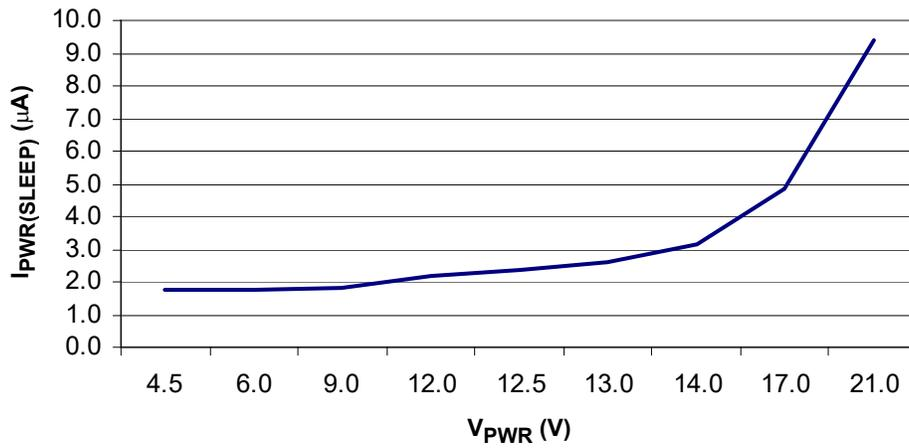
Figure 8. Typical Sleep-state Supply Current vs. V<sub>PWR</sub> at 150 °C
