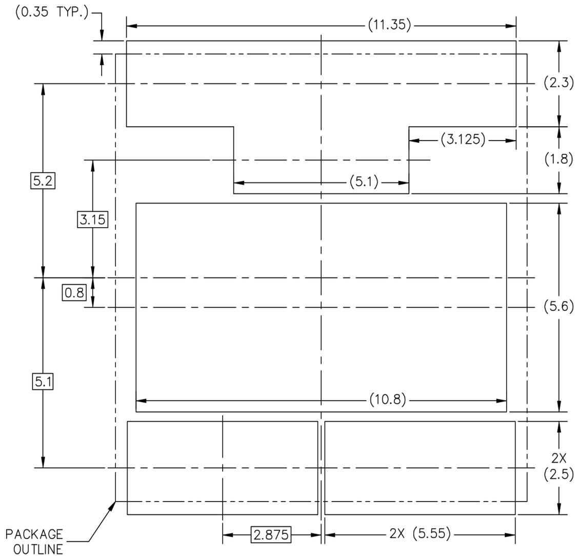
PCB DESIGN GUIDELINES – SOLDER MASK OPENING PATTERN 2
