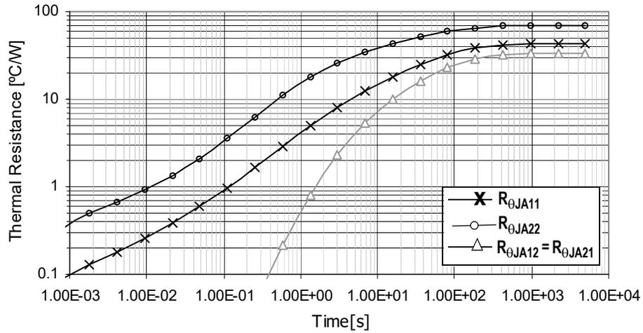
Figure 47. Transient Thermal Resistance R<sub>θJA</sub>,
