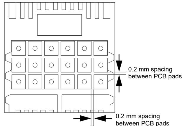
Note: Recommended via diameter is 0.5 mm. PTH (plated through hole) via must be plugged / filled with epoxy or solder mask in order to minimize void formation and to avoid any solder wicking into the via.
