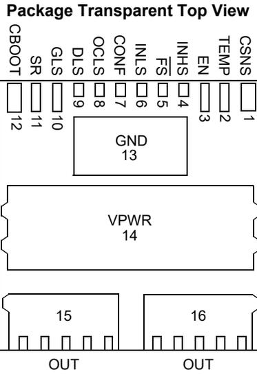
**Figure 3. Pin Connections**
