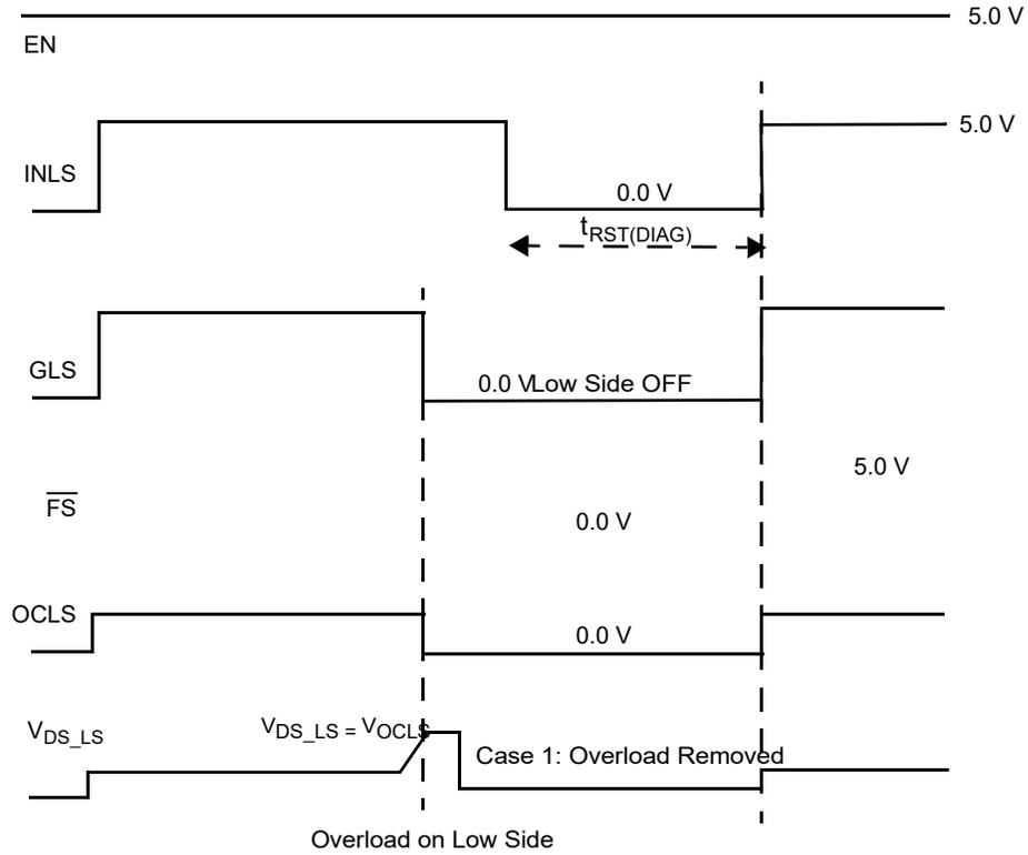
**Figure 13. Overload on Low Side Gate Drive, Case 1**
