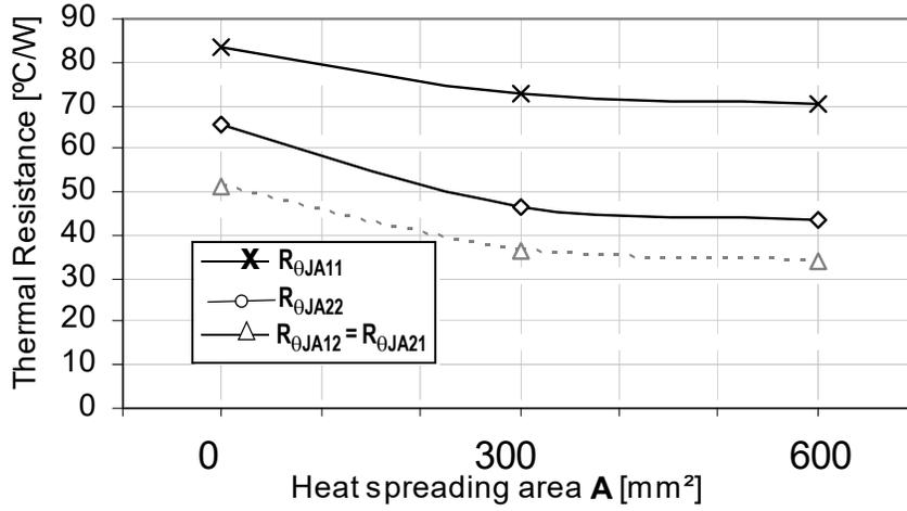
Figure 46. Device on Thermal Test Board R<sub>θJA</sub>
