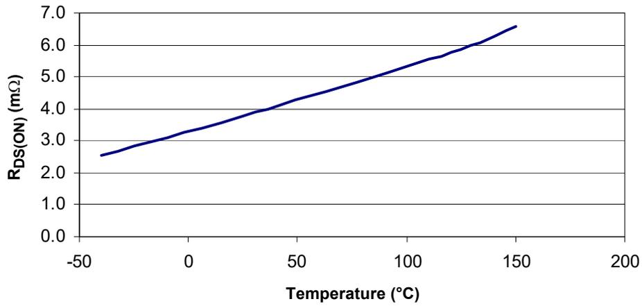
Figure 7. Typical R<sub>DS(ON)</sub> vs. Temperature at V<sub>PWR</sub> = 13 V
