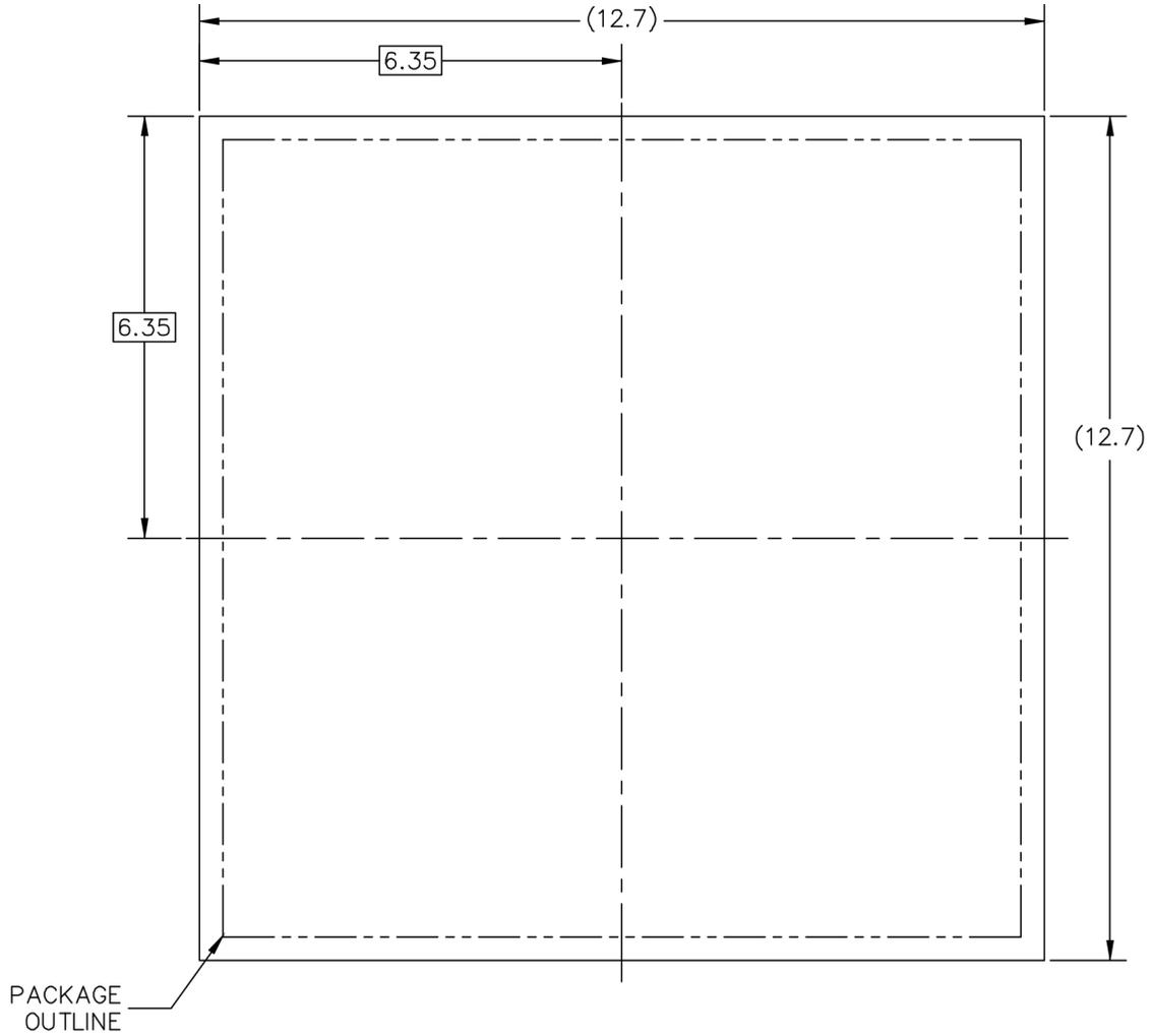
PCB DESIGN GUIDELINES – SOLDER MASK OPENING PATTERN 1
