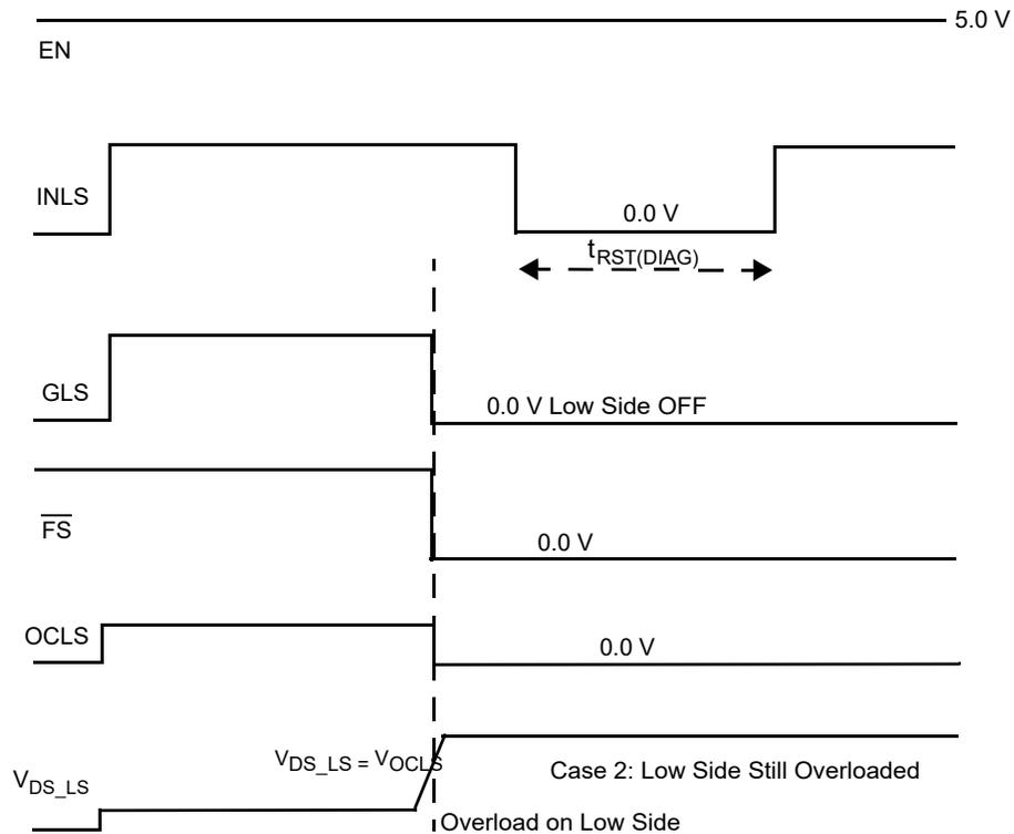
**Figure 14. Overload on Low Side Gate Drive, Case 2**
