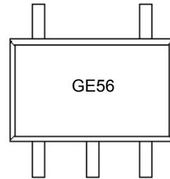
5-Lead SOT-23 (MCP6V96, MCP6V96U)
