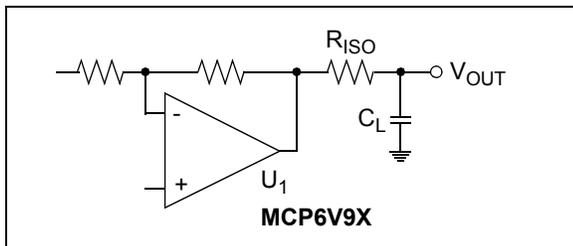
**FIGURE 4-7:** Output Resistor,  $R_{ISO}$ , Stabilizes Capacitive Loads.
