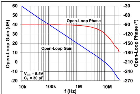
**FIGURE 2-24:** Open-Loop Gain vs. Frequency with  $V_{DD} = 5.5\text{V}$ .
