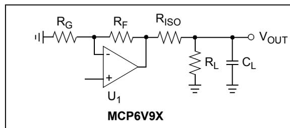
**FIGURE 4-9:** Output Load.
