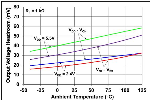
**FIGURE 2-18:** Output Voltage Headroom vs. Ambient Temperature.
