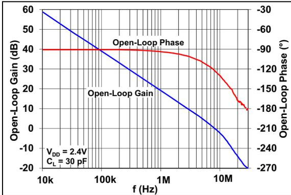
**FIGURE 2-23:** Open-Loop Gain vs. Frequency with  $V_{DD} = 2.4\text{V}$ .
