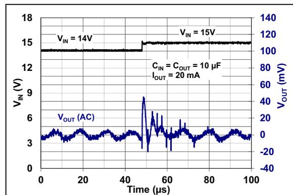
**FIGURE 2-6:** 5V LDO Dynamic Line Step – Rising  $V_{\text{DD}}$ .
