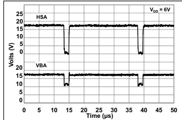
**FIGURE 2-4:** Bootstrap Voltage at 92% Duty Cycle.
