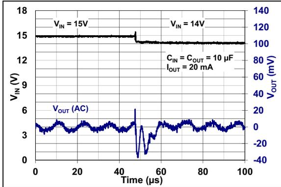
**FIGURE 2-7:** 5V LDO Dynamic Line Step – Falling  $V_{DD}$ .
