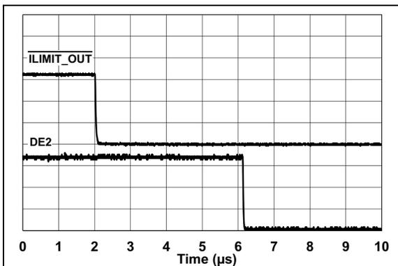
**FIGURE 2-3:**  $\overline{\text{ILIMIT\_OUT}}$  Low to DE2 Message Delay.
