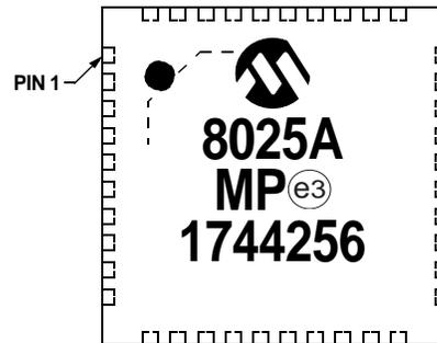
48-Lead TQFP (7x7x1 mm)
