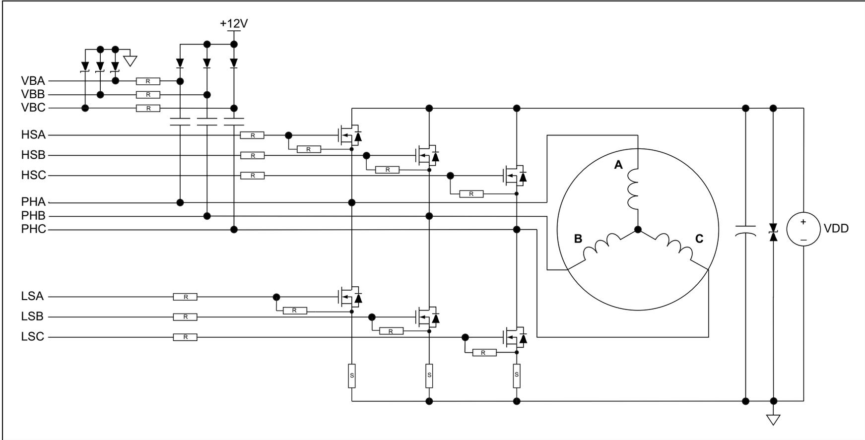
FIGURE 5-3: Overvoltage Protection.
