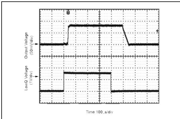
**FIGURE 2-9:** PWM Mode to LDO Mode Transition.
