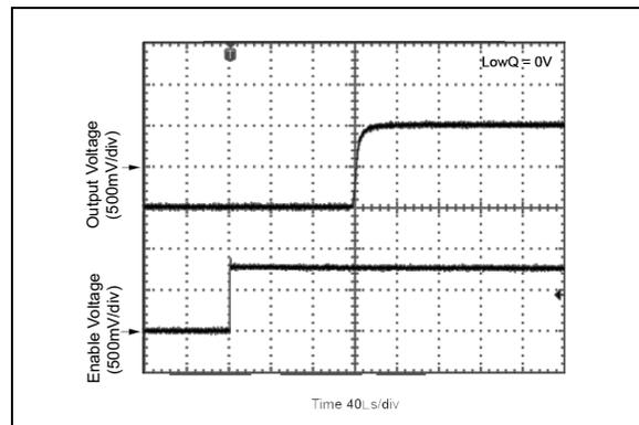
**FIGURE 2-22:** Enable Transient LDO Mode.
