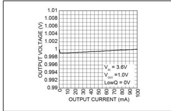
**FIGURE 2-21:** Output Voltage vs. Output Current.
