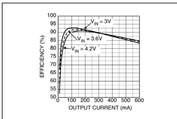
**FIGURE 2-2:** 1.8  $V_{OUT}$  Efficiency.
