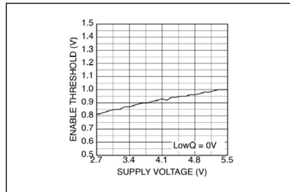
**FIGURE 2-16:** Enable Threshold Voltage vs. Supply Voltage.
