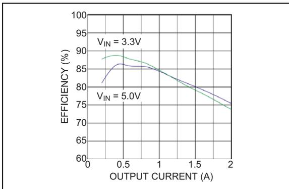
FIGURE 5-1: Efficiency Curve.
