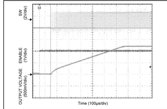
**FIGURE 2-16:** Enable Turn-On.
