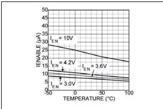
**FIGURE 2-8:** EN Pin Bias Current vs. Temperature.
