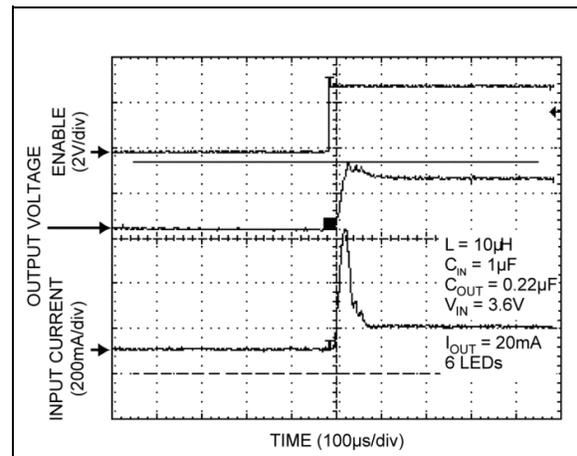
**FIGURE 2-16:** 6-Series LED Circuit without External Soft-Start.
