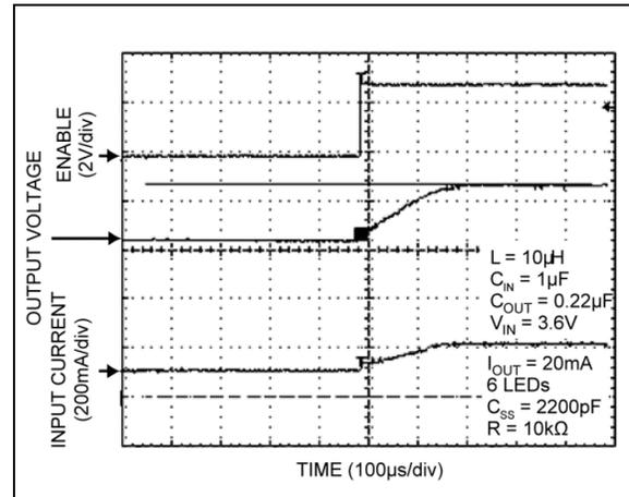
**FIGURE 2-15:** 6-Series LED Circuit with External Soft-Start.
