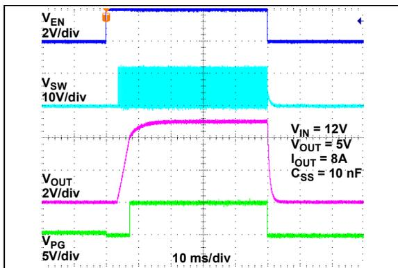
FIGURE 2-44: Enable Turn-On/Turn-Off.
