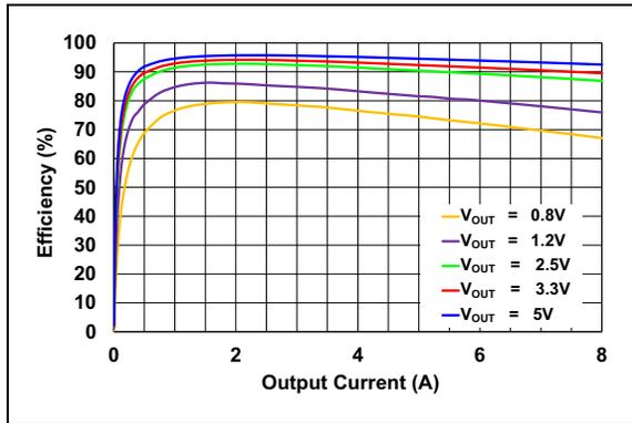
**FIGURE 2-1:** Efficiency vs. Output Current ( $V_{IN} = 12V$ ).
