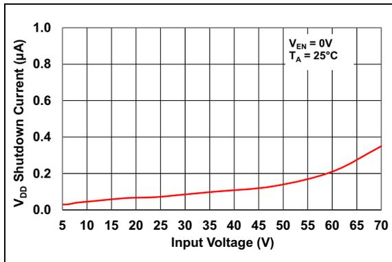
**FIGURE 2-26:**  $V_{DD}$  Shutdown Current vs. Input Voltage.
