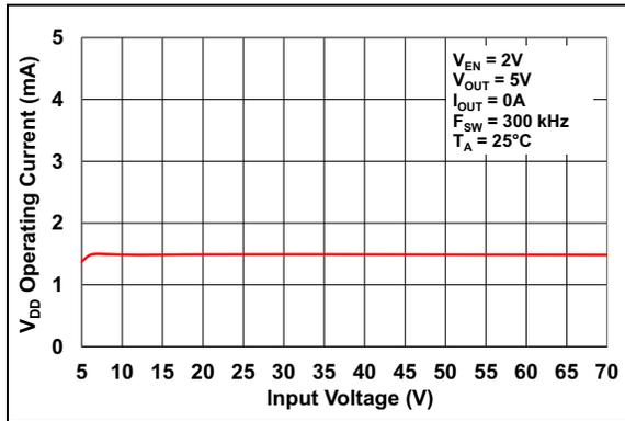
**FIGURE 2-25:**  $V_{DD}$  Operating Current vs. Input Voltage.
