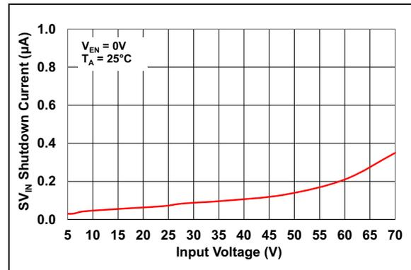
**FIGURE 2-29:**  $SV_{IN}$  Shutdown Current vs. Input Voltage.
