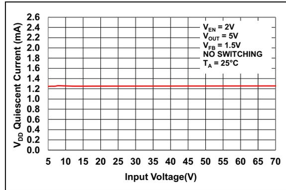
**FIGURE 2-23:**  $V_{DD}$  Quiescent Current vs. Input Voltage.
