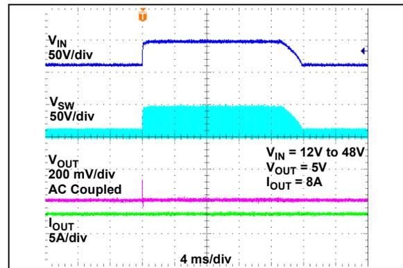
**FIGURE 2-64:** Line Transient Response ( $V_{IN} = 12V$  to  $48V$ ).
