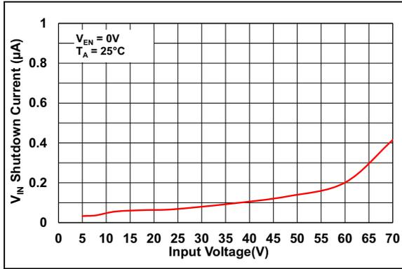
**FIGURE 2-19:**  $V_{IN}$  Shutdown Current vs. Input Voltage.
