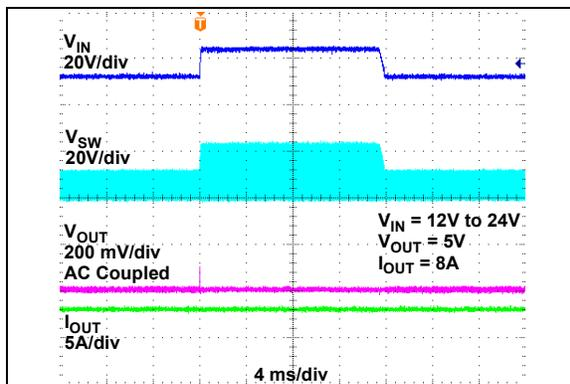
**FIGURE 2-62:** Line Transient Response ( $V_{IN} = 12V$  to  $24V$ ).
