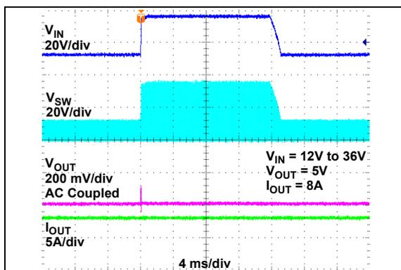
**FIGURE 2-63:** Line Transient Response ( $V_{IN} = 12V$  to  $36V$ ).
