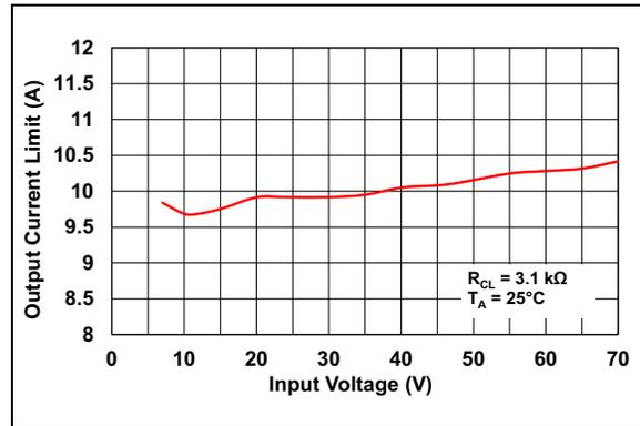
**FIGURE 2-34:** Output Current Limit vs. Input Voltage.
