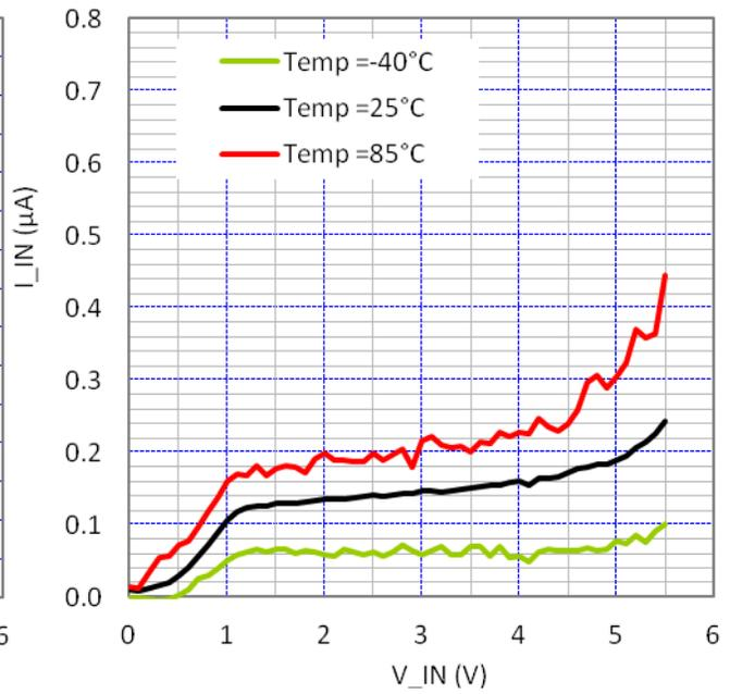
Figure 9. Standby Current ( $\mu\text{A}$ ) vs. Temperature ( $^{\circ}\text{C}$ )
