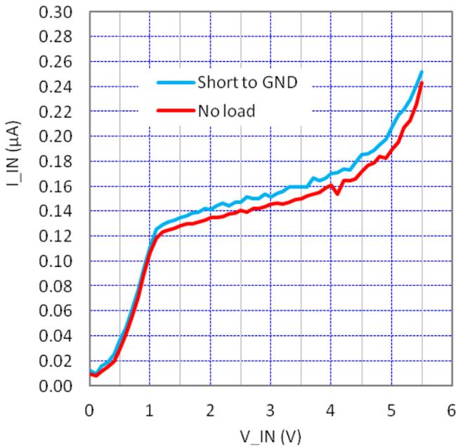
Figure 8. Standby ( $\mu\text{A}$ ) and Leakage Current ( $\mu\text{A}$ ) vs.  $V_{\text{in}}$  (V)
