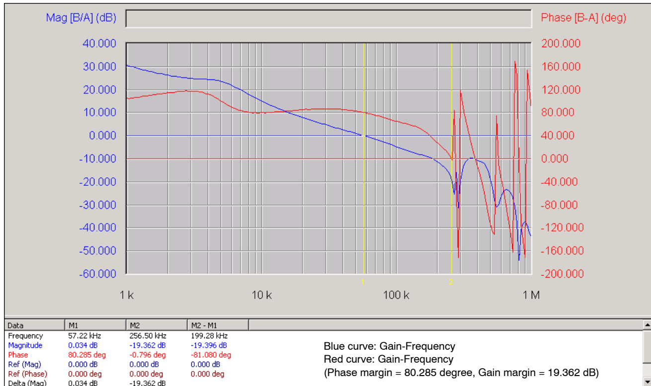
Figure 14. Closed-loop Voltage Loop-gain of the NCP81044
