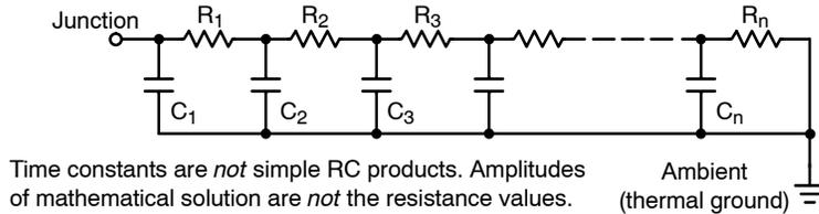
**Figure 12. Grounded Capacitor Thermal Network (“Cauer” Ladder)**
