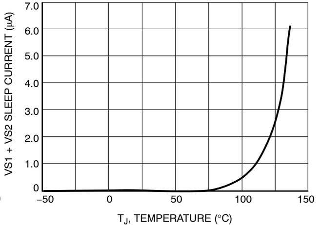
Figure 9. VS1 + VS2 Sleep Current vs. Temperature
