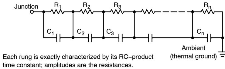
**Figure 13. Non-Grounded Capacitor Thermal Ladder (“Foster” Ladder)**
