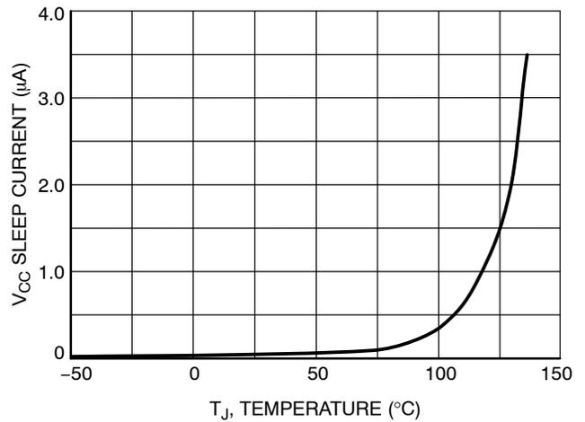
Figure 7. VCC Sleep Supply Current vs. Temperature
