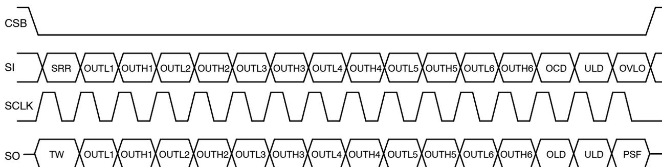
**Figure 3. SPI Communication Frame Format**
