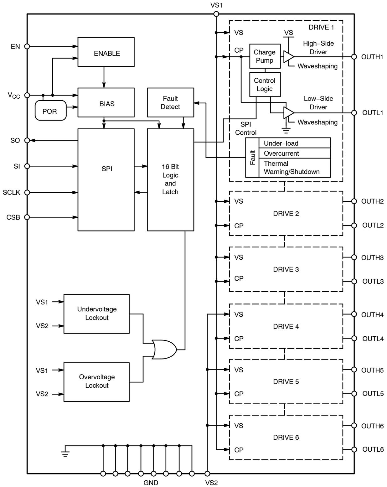
Figure 1. Block Diagram
