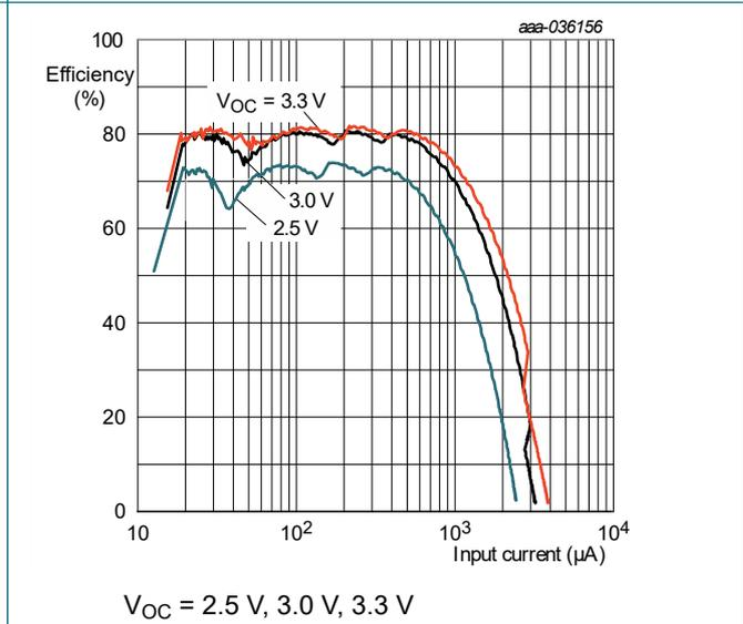
Fig. 11. Efficiency as a function of input current
