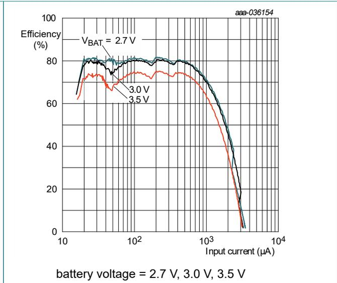
Fig. 9. Efficiency as a function of input current
