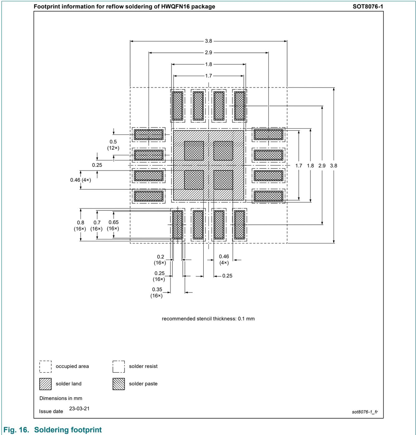
Fig. 16. Soldering footprint
