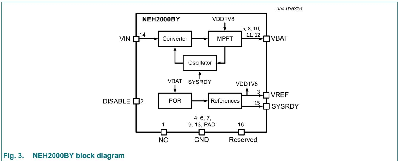
Fig. 3. NEH2000BY block diagram
