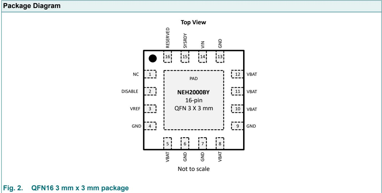
Fig. 2. QFN16 3 mm x 3 mm package
