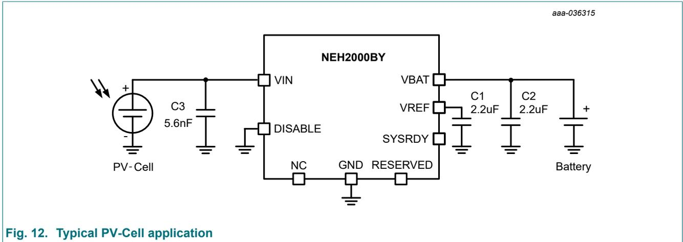
Fig. 12. Typical PV-Cell application
