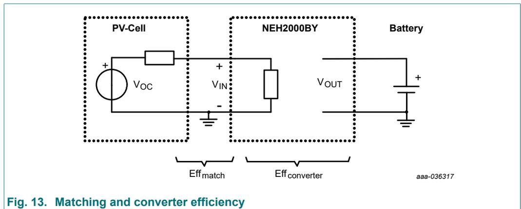
Fig. 13. Matching and converter efficiency
