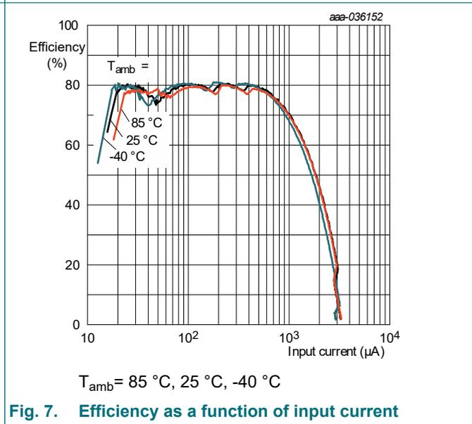
$V_{BAT} = 3\text{ V}$ ,  $V_{OC} = 3\text{ V}$ ,  $T_{amb} = 25\text{ }^{\circ}\text{C}$ , unless otherwise specified.
