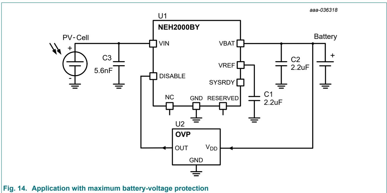
Fig. 14. Application with maximum battery-voltage protection
