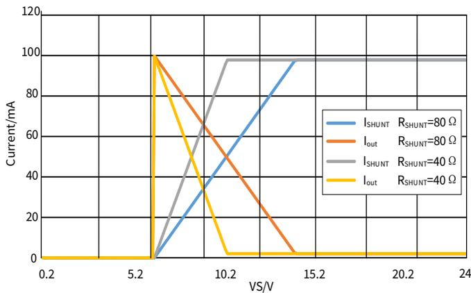
Figure 6.11 Output Current Distribution vs Supply Voltage ( $I_{set}=99mA$ )
