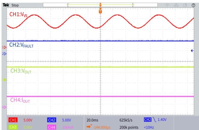
Figure 6.9 Superimposed Alternating Voltage 15Hz
