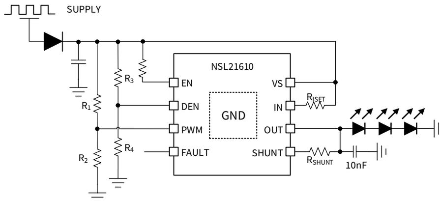
Figure 7.4 NSL21610 Power Supply Control LED Brightness Dimming
