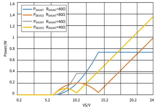
Figure 6.12 Power Dissipation vs Supply Voltage ( $I_{set}=99mA$ )
