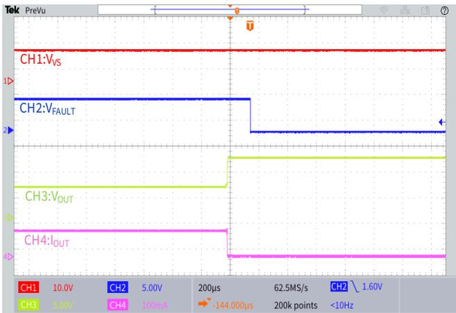
Figure 6.5 Open-Load Protection
