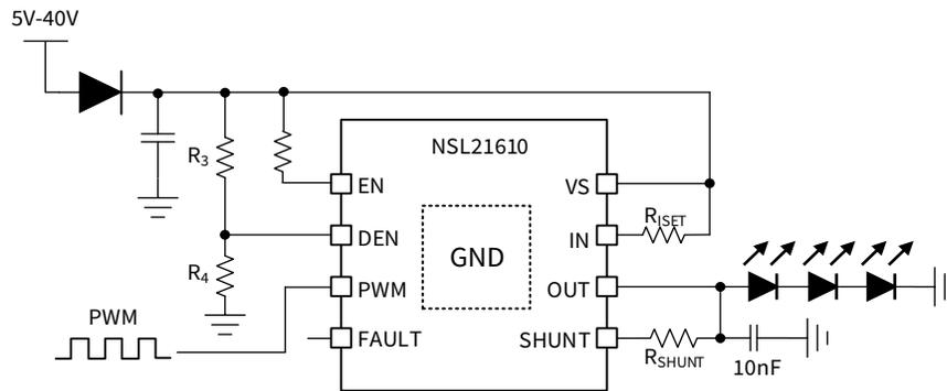
Figure 7.3 NSL21610 PWM Control LED Brightness Dimming
