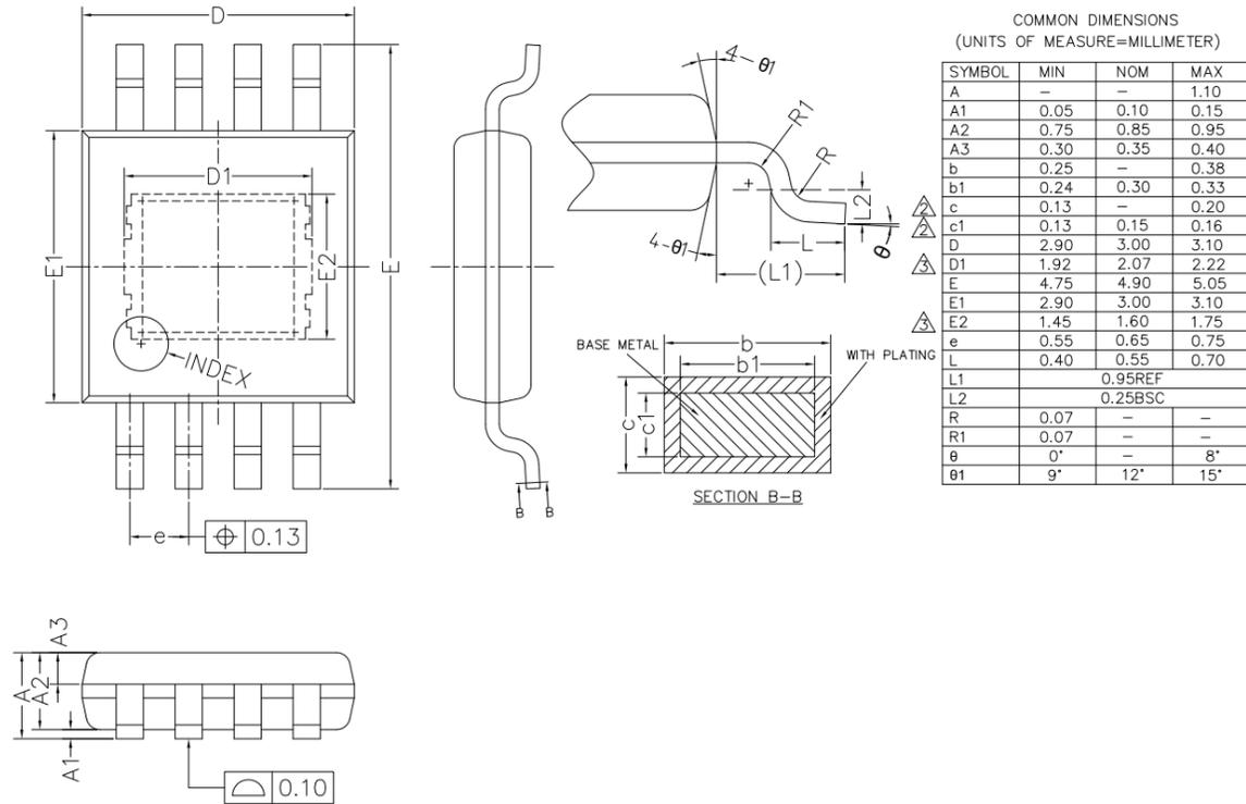
Figure 10.1 HMSOP-8 Package Shape and Dimension in millimeters
