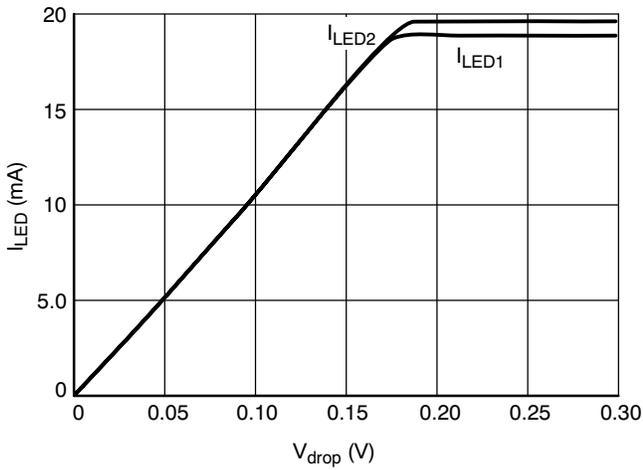
Figure 5. Typical Current Regulation vs.  $V_{drop}$
