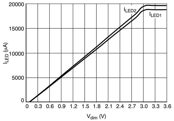
Figure 6. Typical Current Regulation vs.  $V_{dim}$
