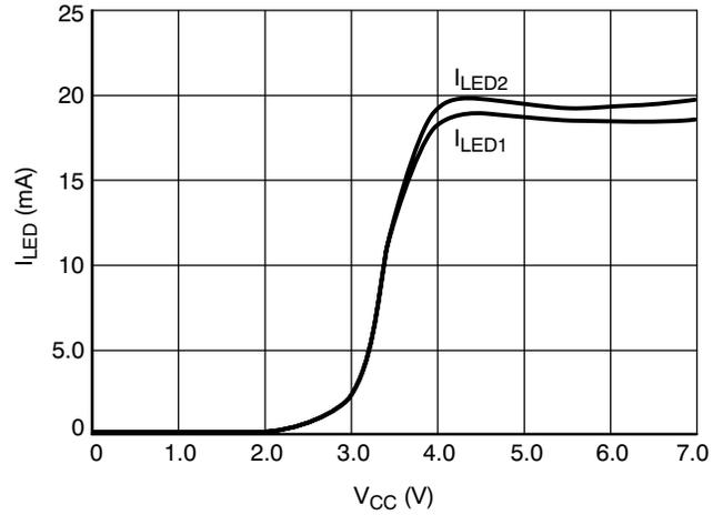
Figure 4. Typical Line Regulation Performance
