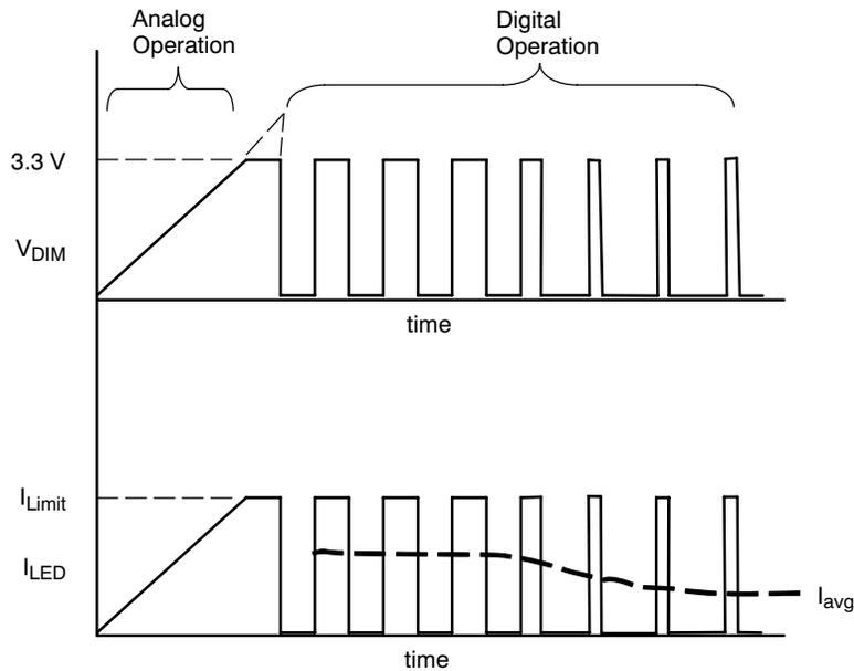
**Figure 7. Dimming Operation Curves**
