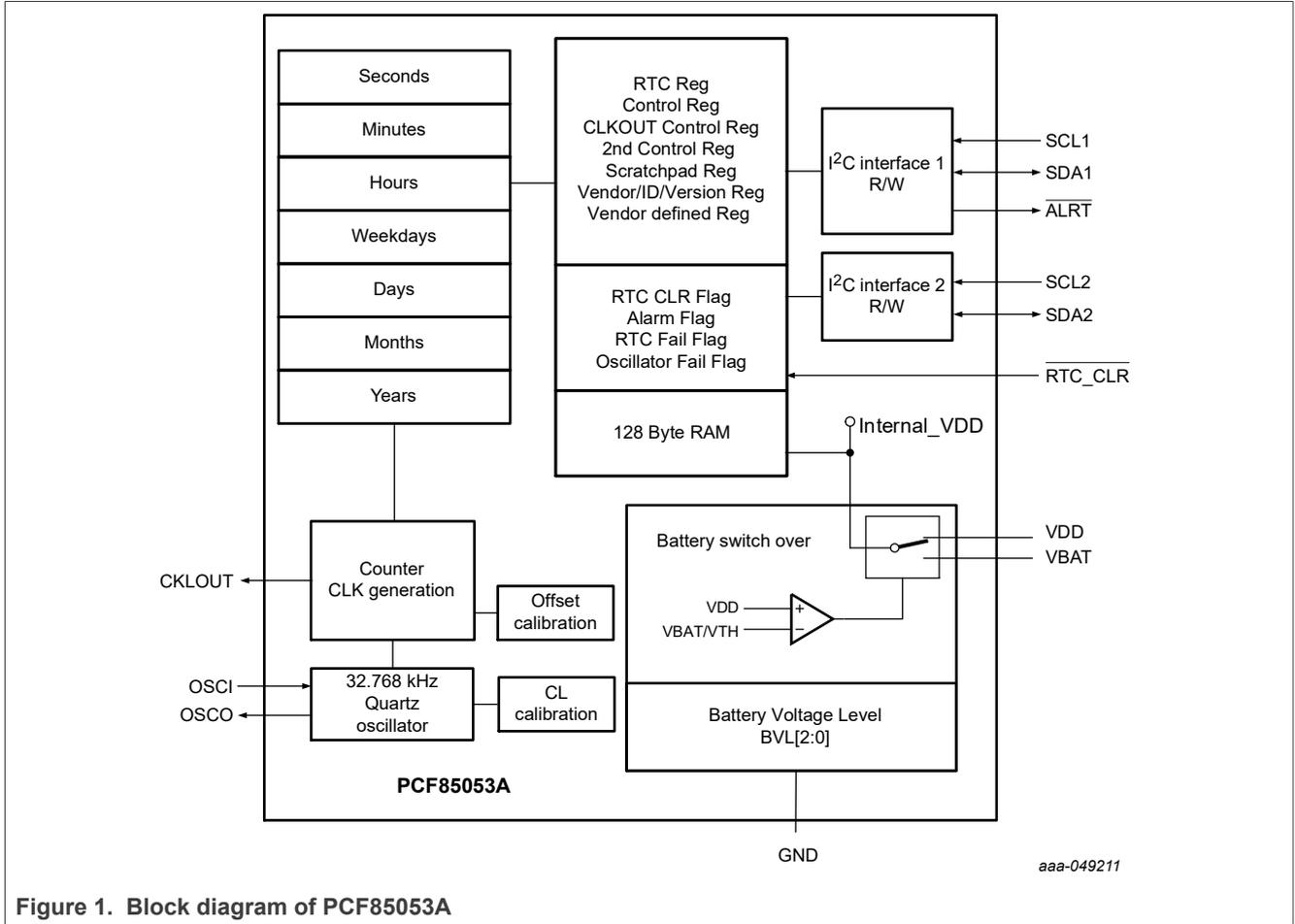
Figure 1. Block diagram of PCF85053A
