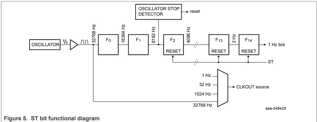
The ST bit function will not affect the output of 32.768 kHz on CLKOUT, but will stop the generation of 1.024 kHz, 32 Hz, and 1 Hz.
