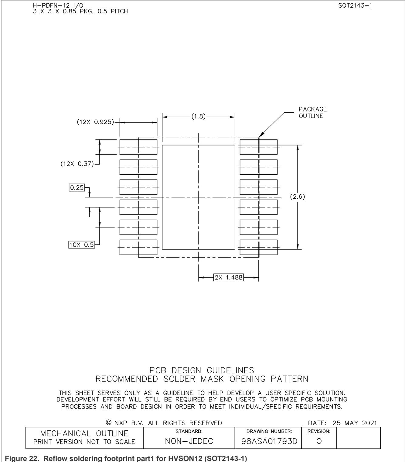
Figure 22. Reflow soldering footprint part1 for HVSON12 (SOT2143-1)
