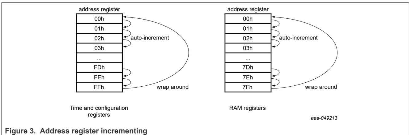
All registers are designed as addressable 8-bit parallel registers although not all bits are implemented.
