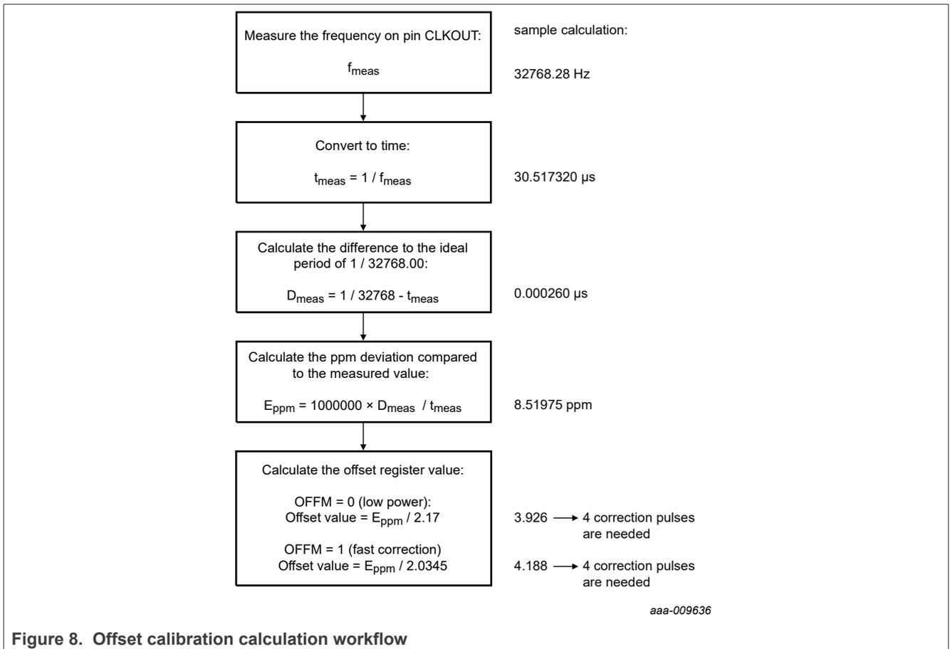
Figure 8. Offset calibration calculation workflow
