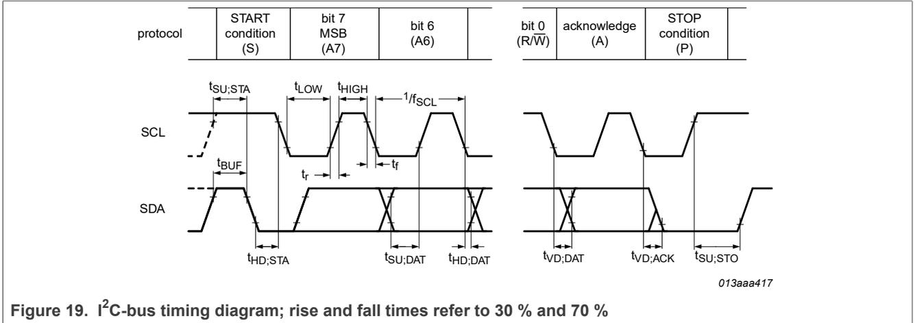
Figure 19. I<sup>2</sup>C-bus timing diagram; rise and fall times refer to 30 % and 70 %
