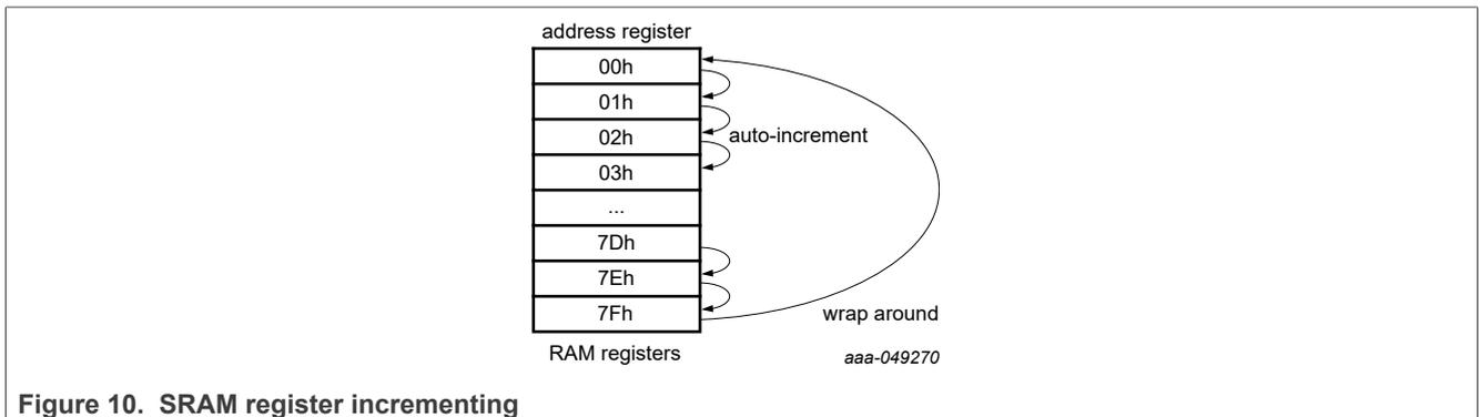
Figure 10. SRAM register incrementing
