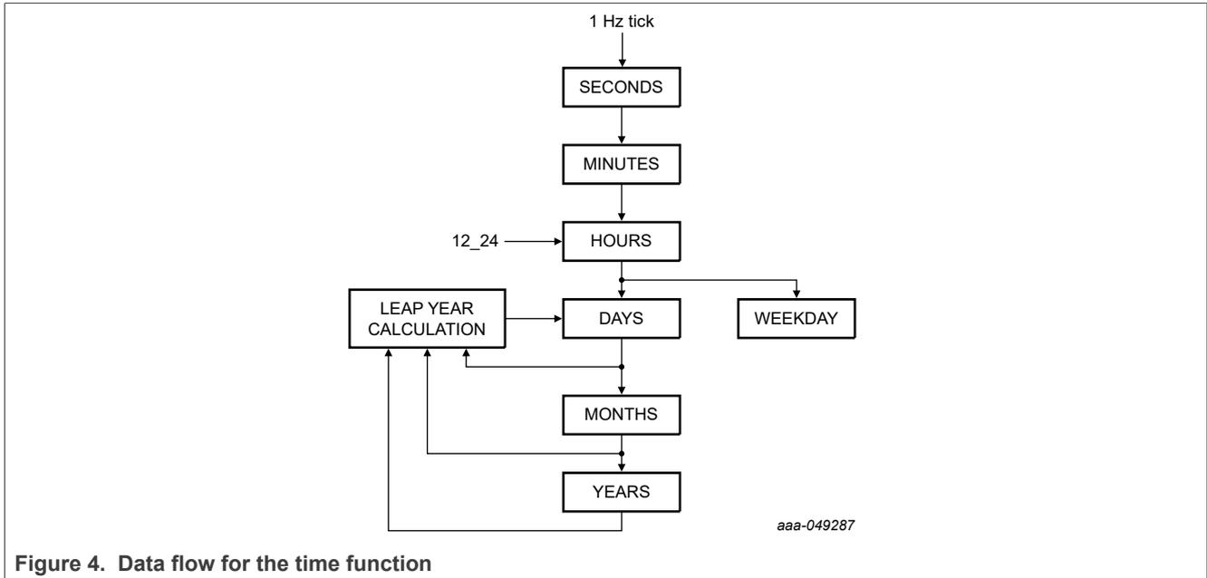
Figure 4. Data flow for the time function
