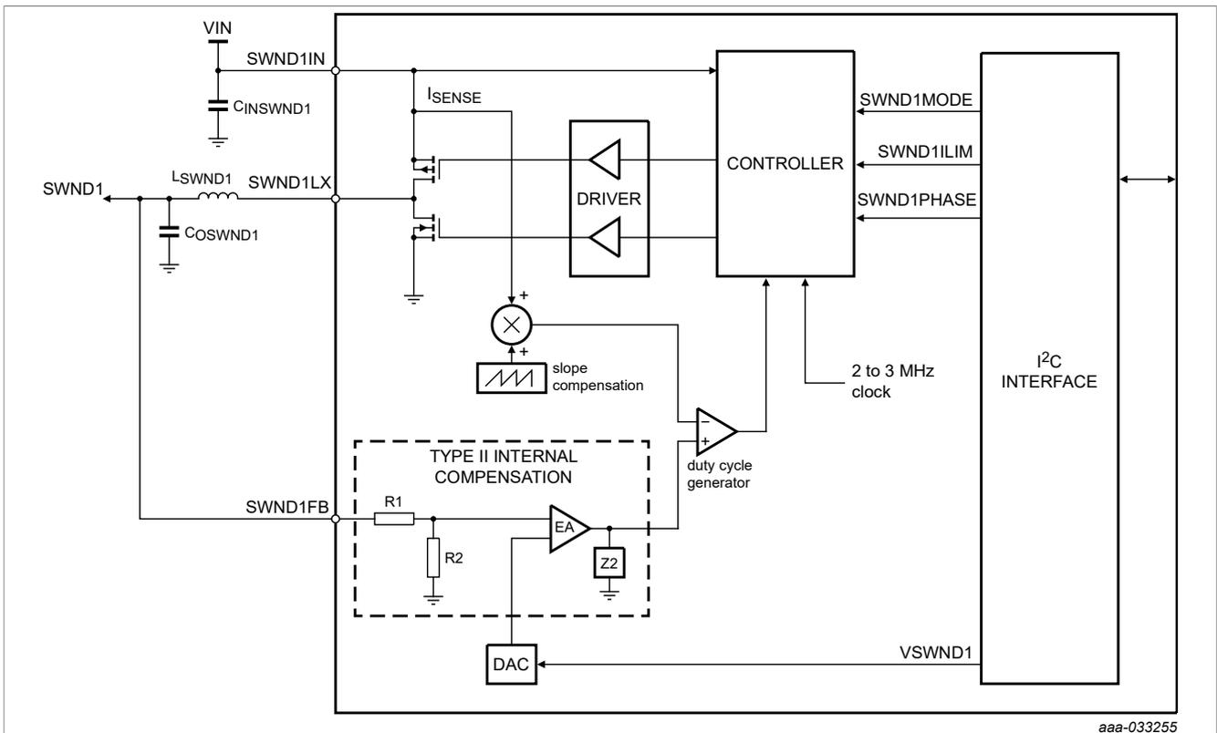
Figure 25. Type 2 buck regulator block diagram
