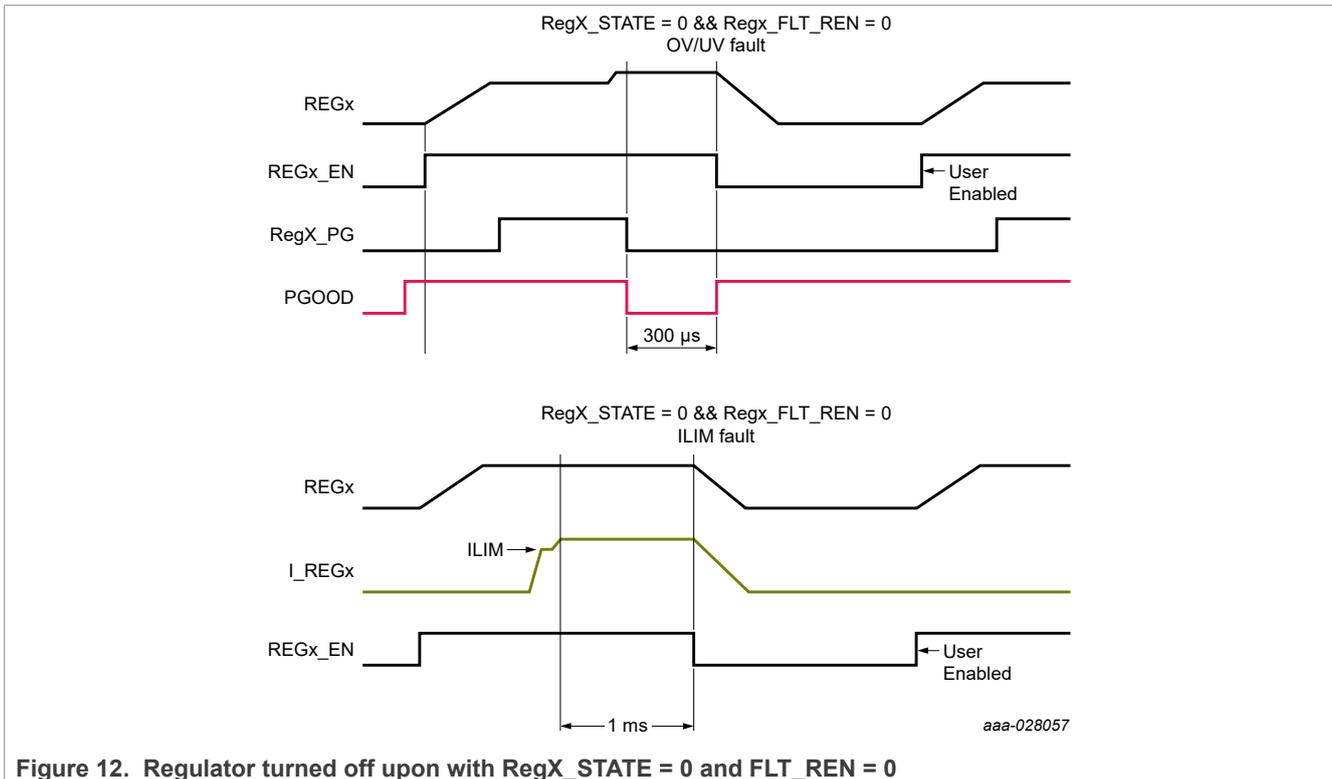
Figure 12. Regulator turned off upon with RegX\_STATE = 0 and FLT\_REN = 0
