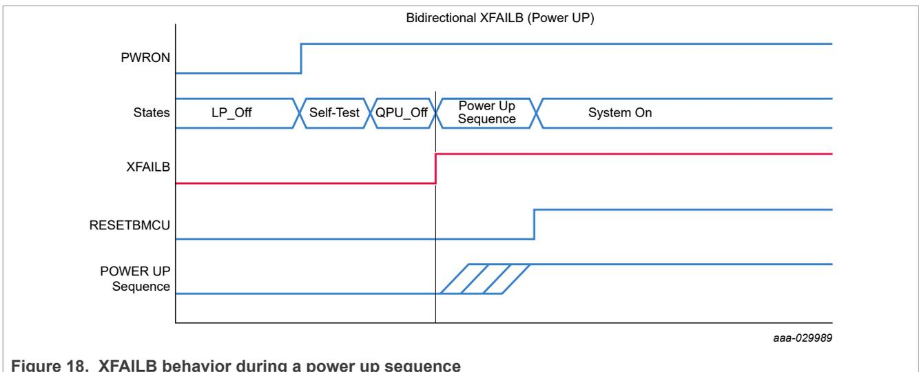
Figure 18. XFAILB behavior during a power up sequence
