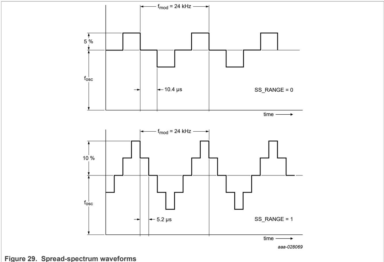
Figure 29. Spread-spectrum waveforms
