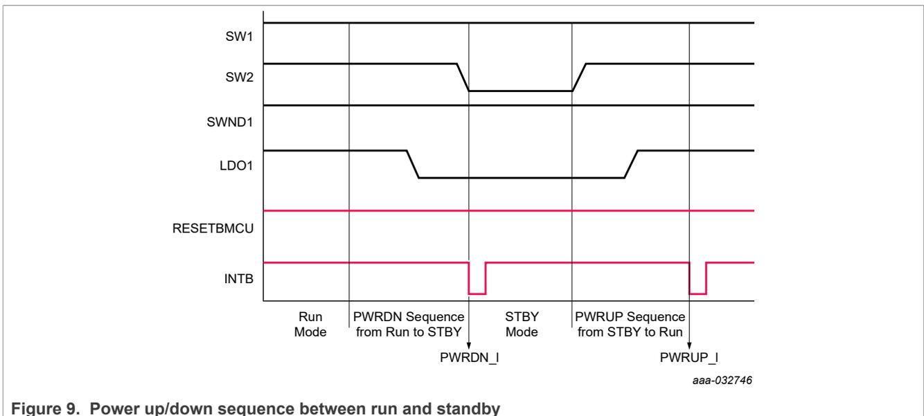
Figure 9. Power up/down sequence between run and standby
