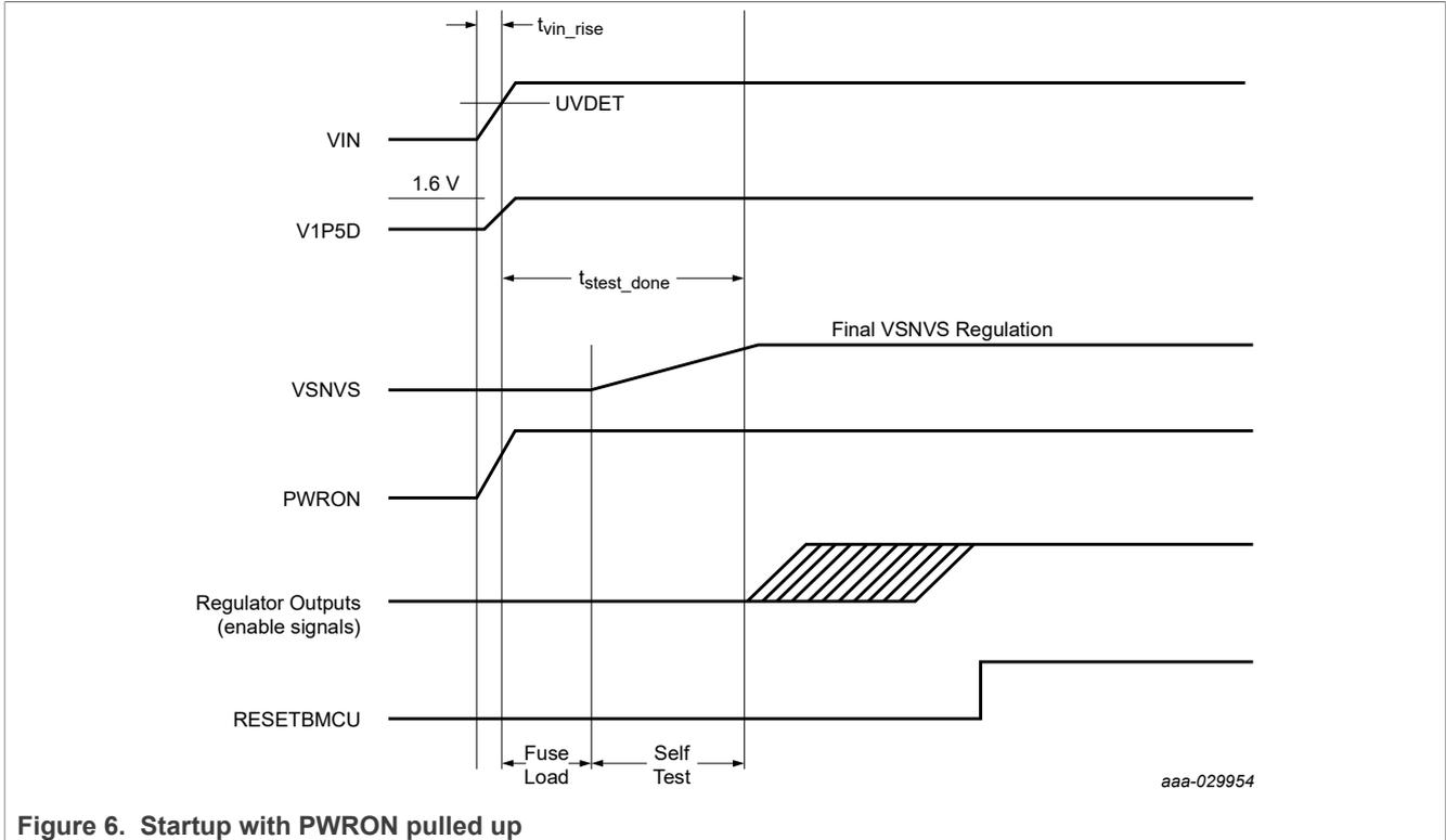
Figure 6. Startup with PWRON pulled up
