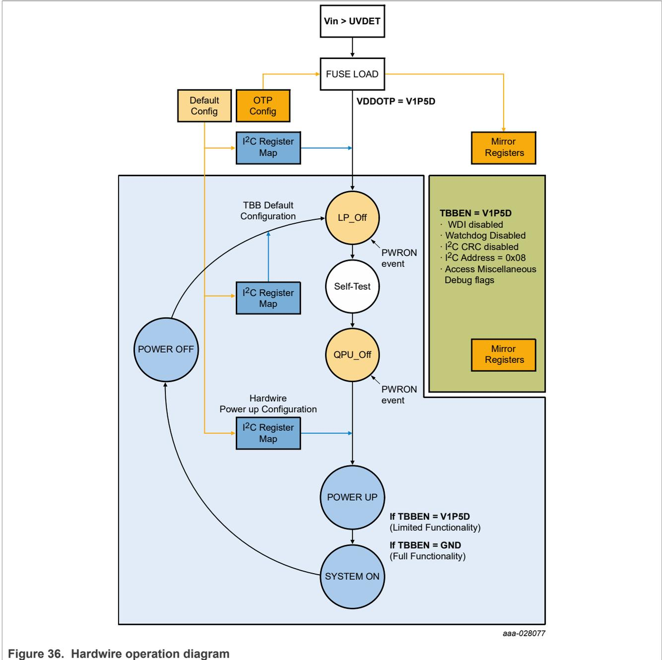
Figure 36. Hardware operation diagram
