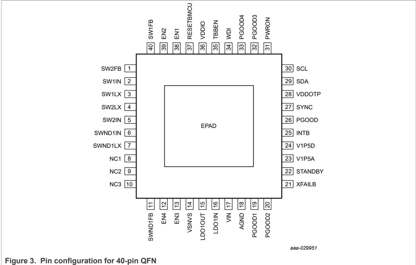
Figure 3. Pin configuration for 40-pin QFN
