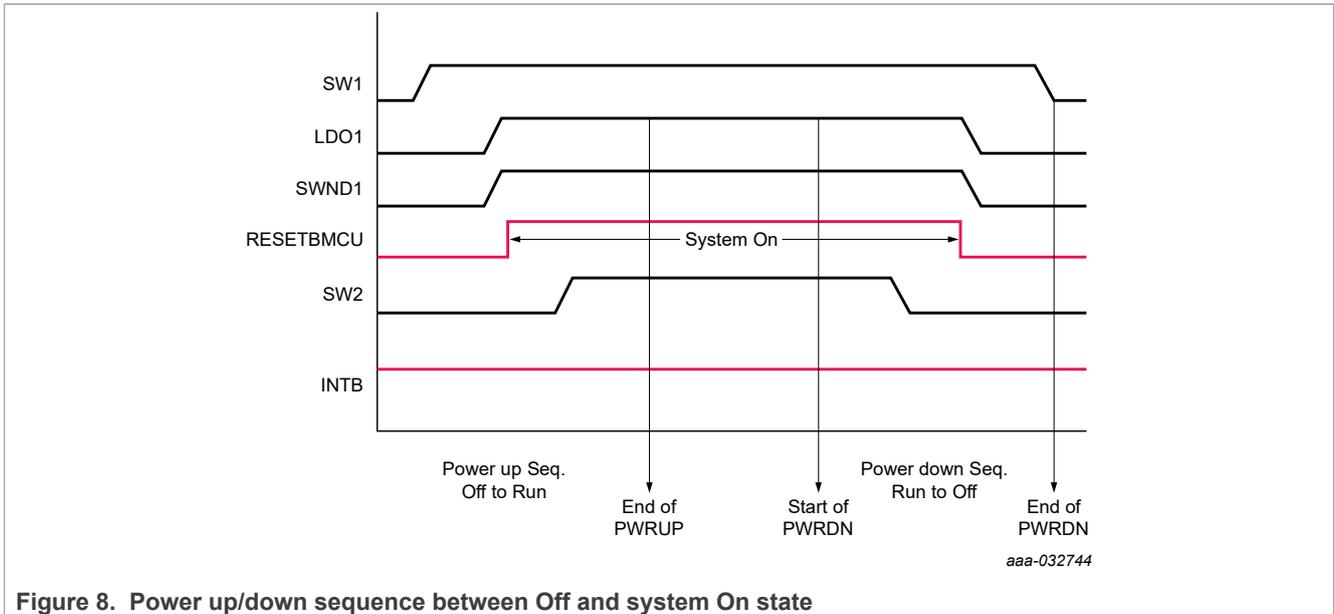
Figure 8. Power up/down sequence between Off and system On state
