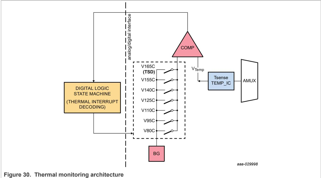
Figure 30. Thermal monitoring architecture
