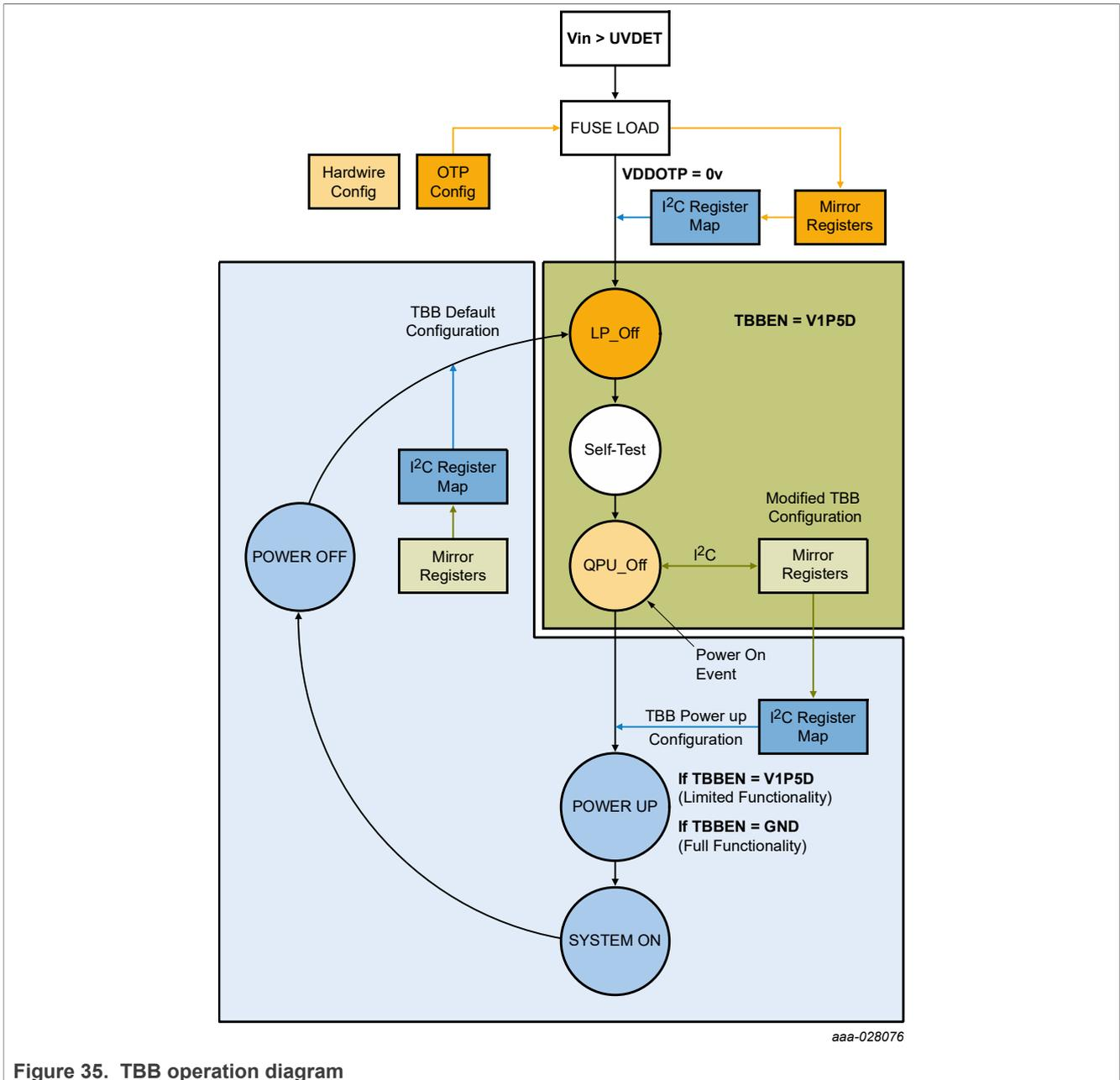
Figure 35. TBB operation diagram
