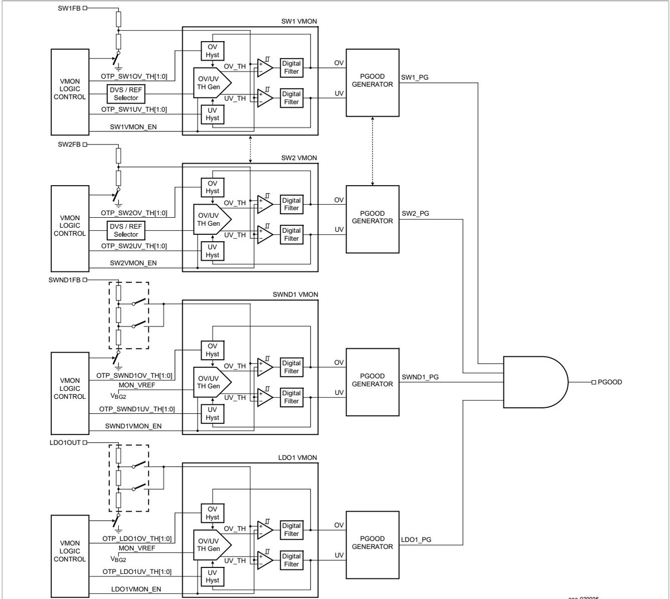
Figure 27. Voltage monitoring architecture
