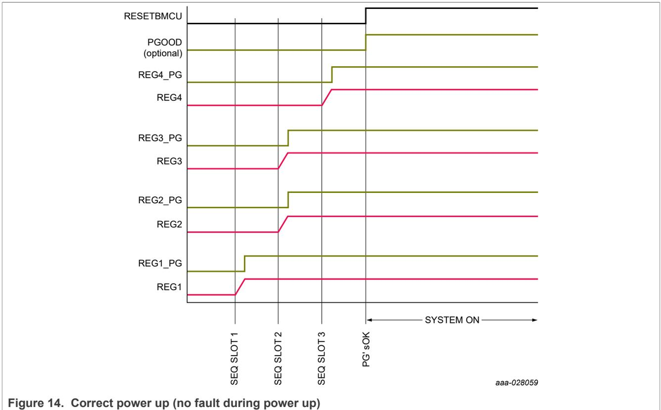
Figure 14. Correct power up (no fault during power up)
