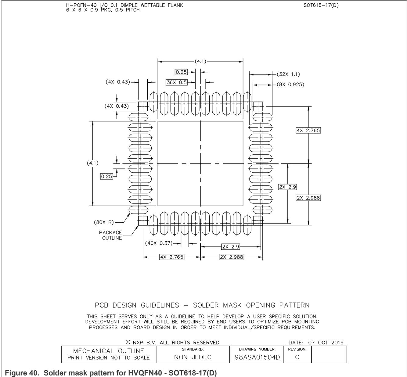
Figure 40. Solder mask pattern for HVQFN40 - SOT618-17(D)
