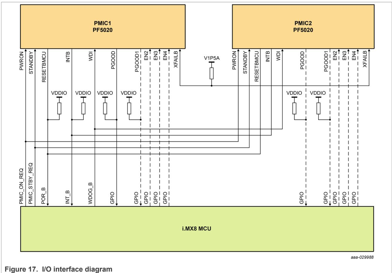
Figure 17. I/O interface diagram
