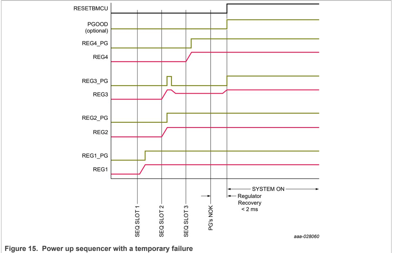
If the faulty condition is not cleared within the 2.0 ms timer, the power up sequence is aborted and the PF5020 turns off all voltage regulators enabled so far as shown in [Figure 16](#).
