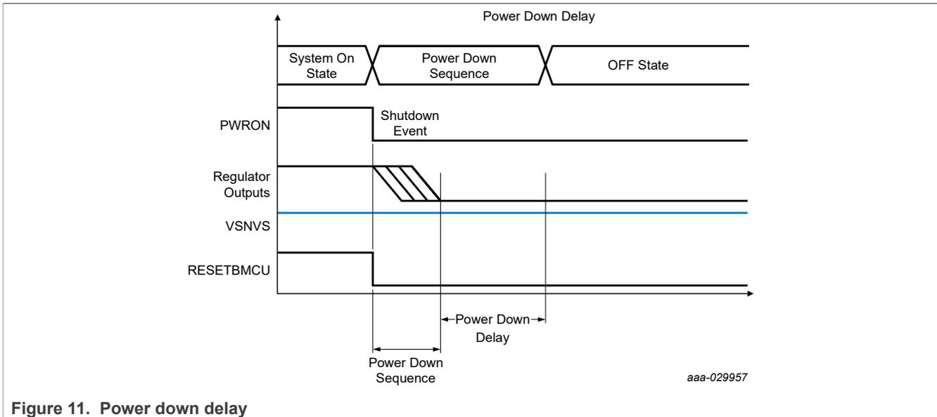
Figure 11. Power down delay
