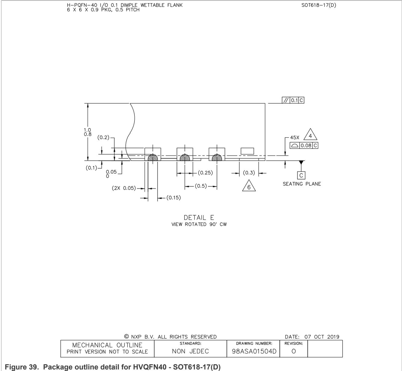
Figure 39. Package outline detail for HVQFN40 - SOT618-17(D)
