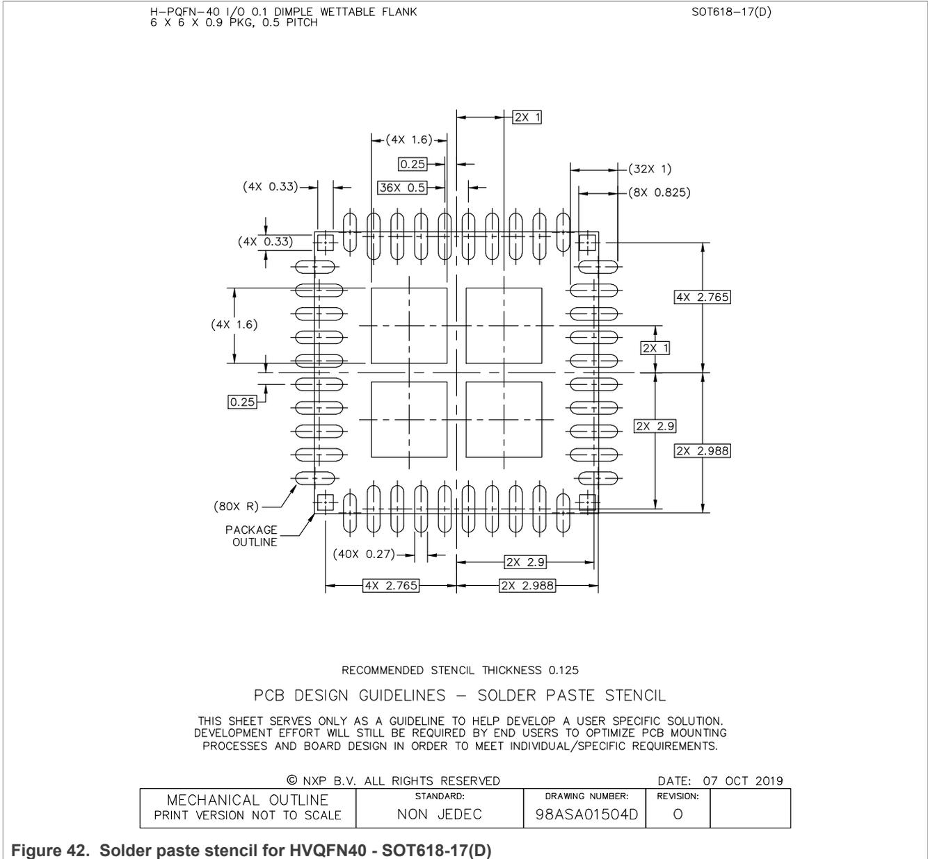
Figure 42. Solder paste stencil for HVQFN40 - SOT618-17(D)
