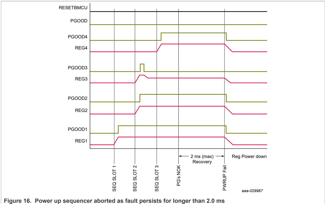
Figure 16. Power up sequencer aborted as fault persists for longer than 2.0 ms
