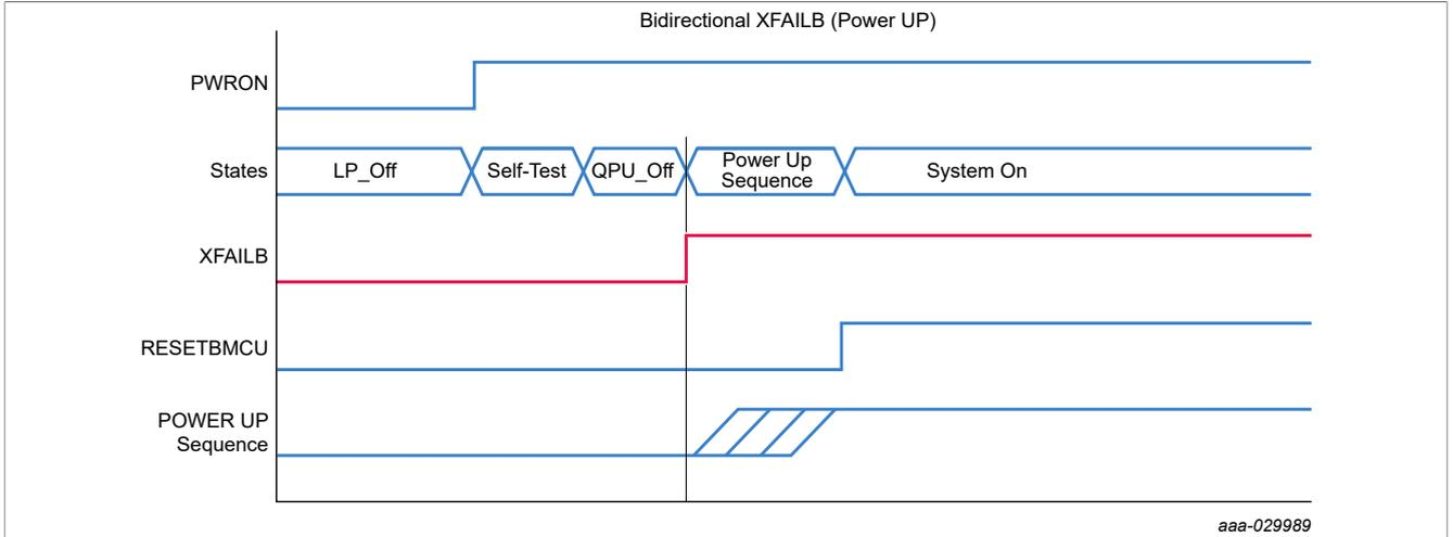
Figure 18. XFAILB behavior during a power up sequence
