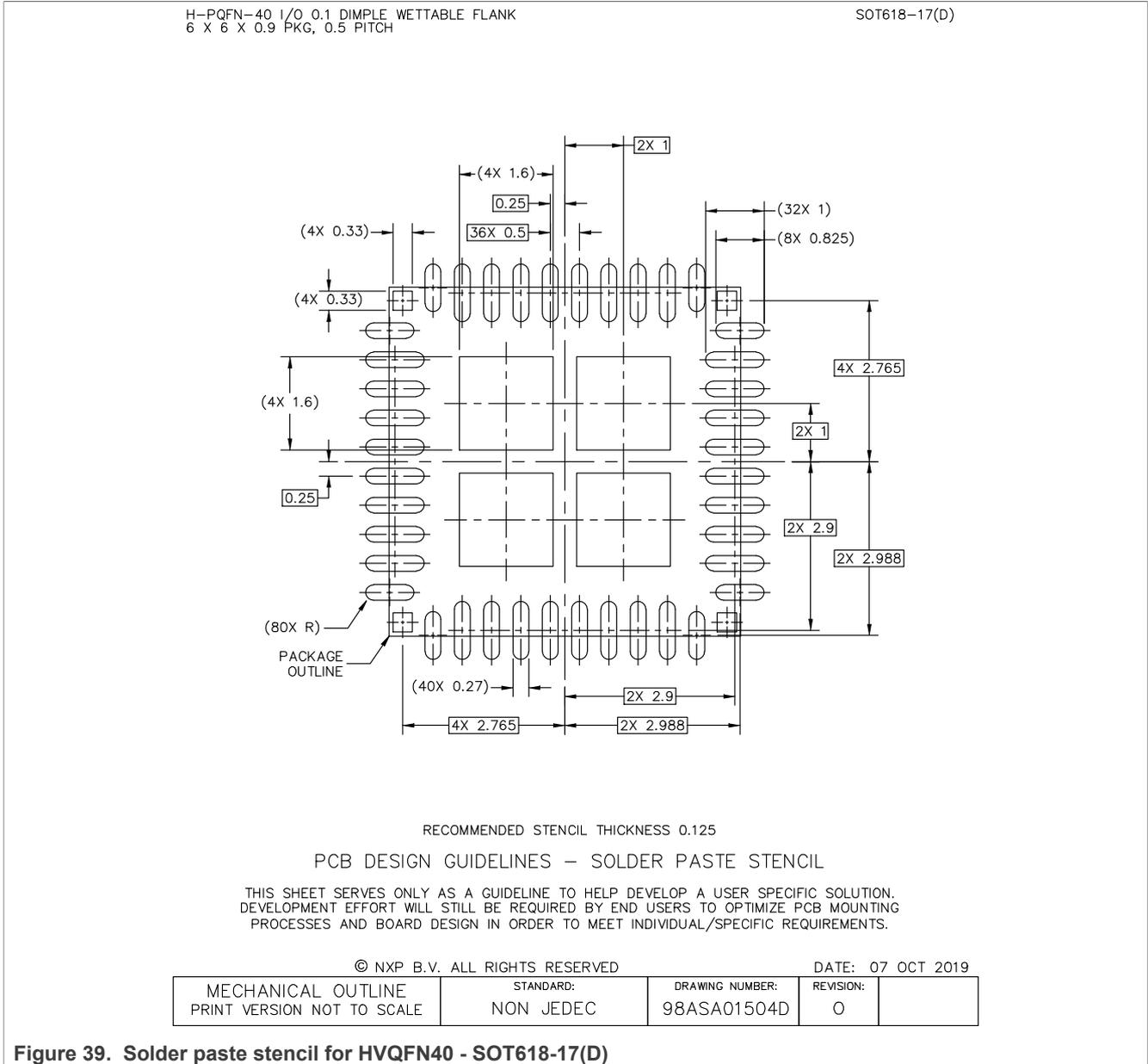
Figure 39. Solder paste stencil for HVQFN40 - SOT618-17(D)
