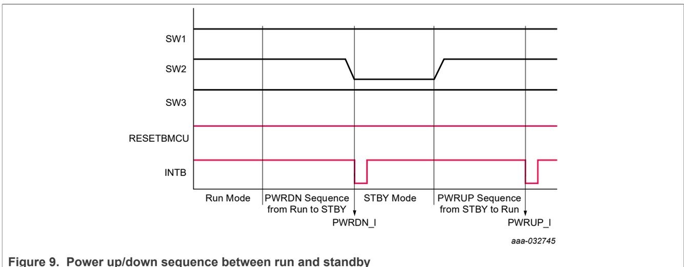
Figure 9. Power up/down sequence between run and standby
