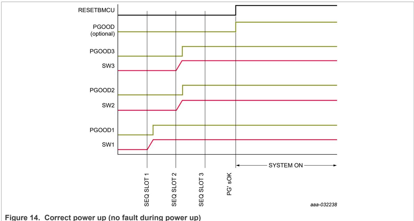
Figure 14. Correct power up (no fault during power up)
