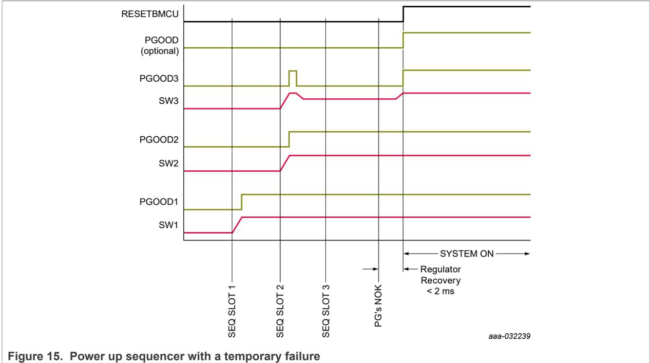
Figure 15. Power up sequencer with a temporary failure
