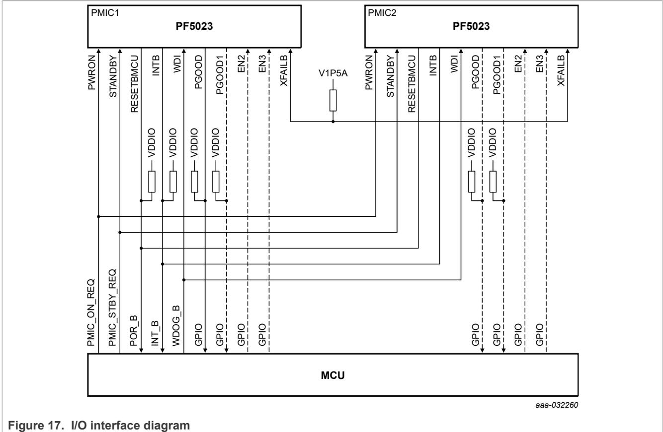
Figure 17. I/O interface diagram
