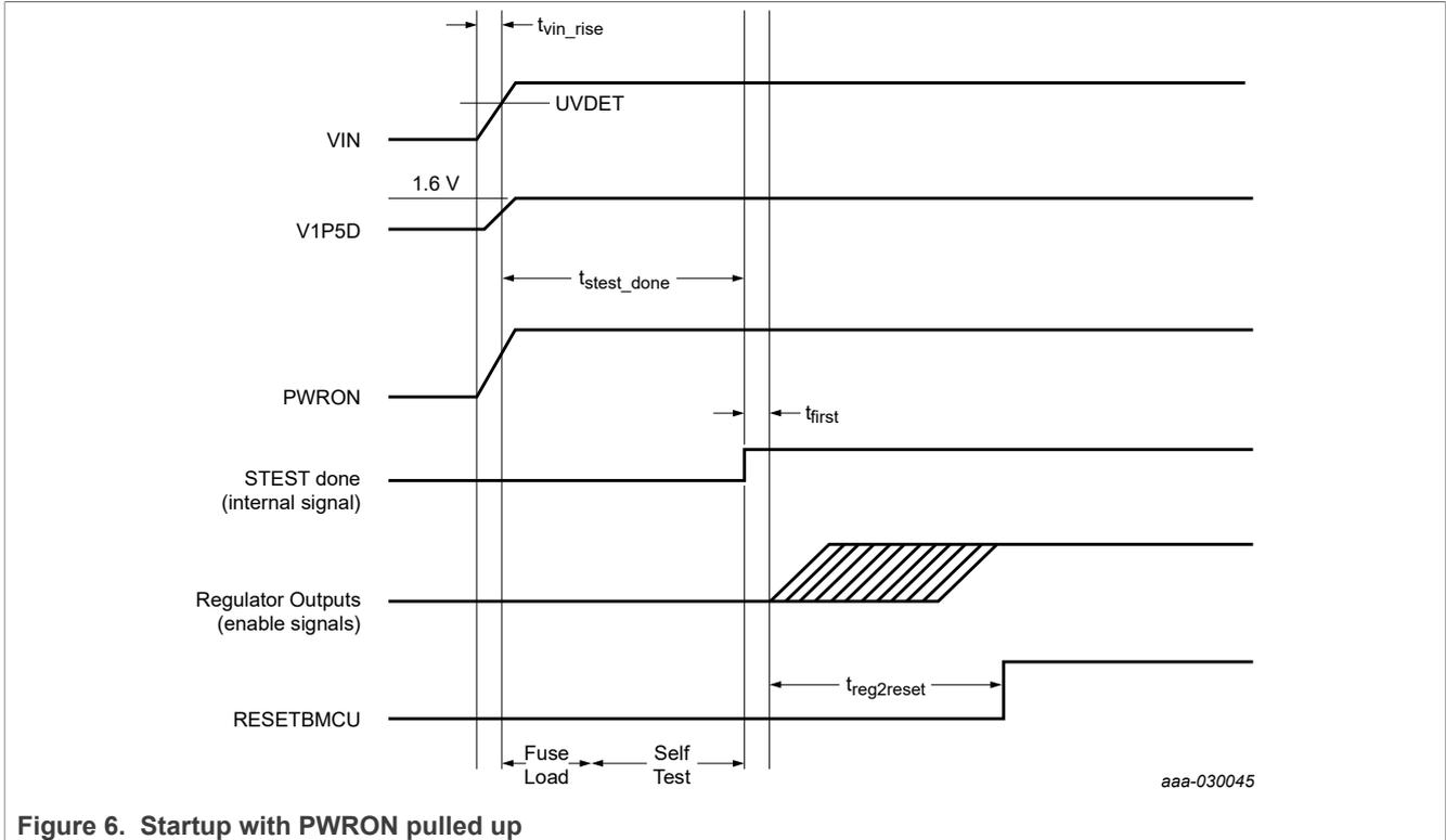
Figure 6. Startup with PWRON pulled up
