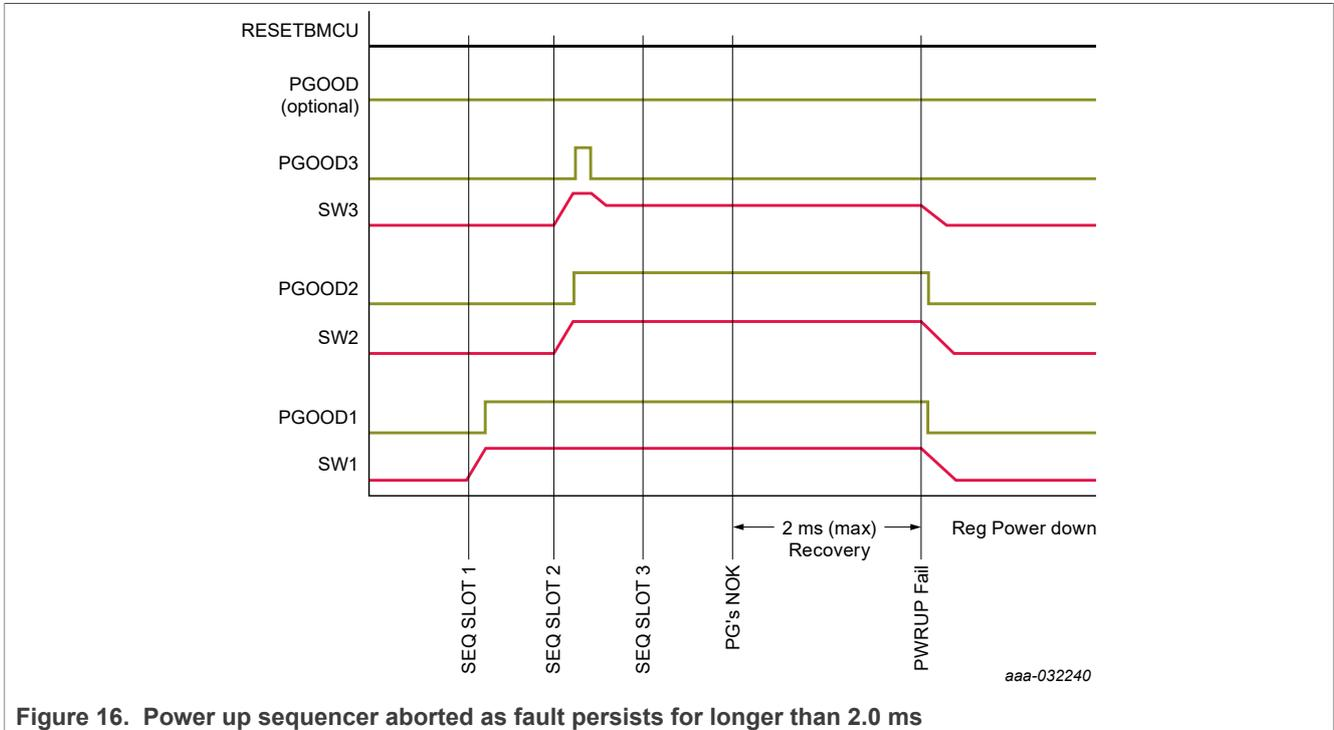
Figure 16. Power up sequencer aborted as fault persists for longer than 2.0 ms
