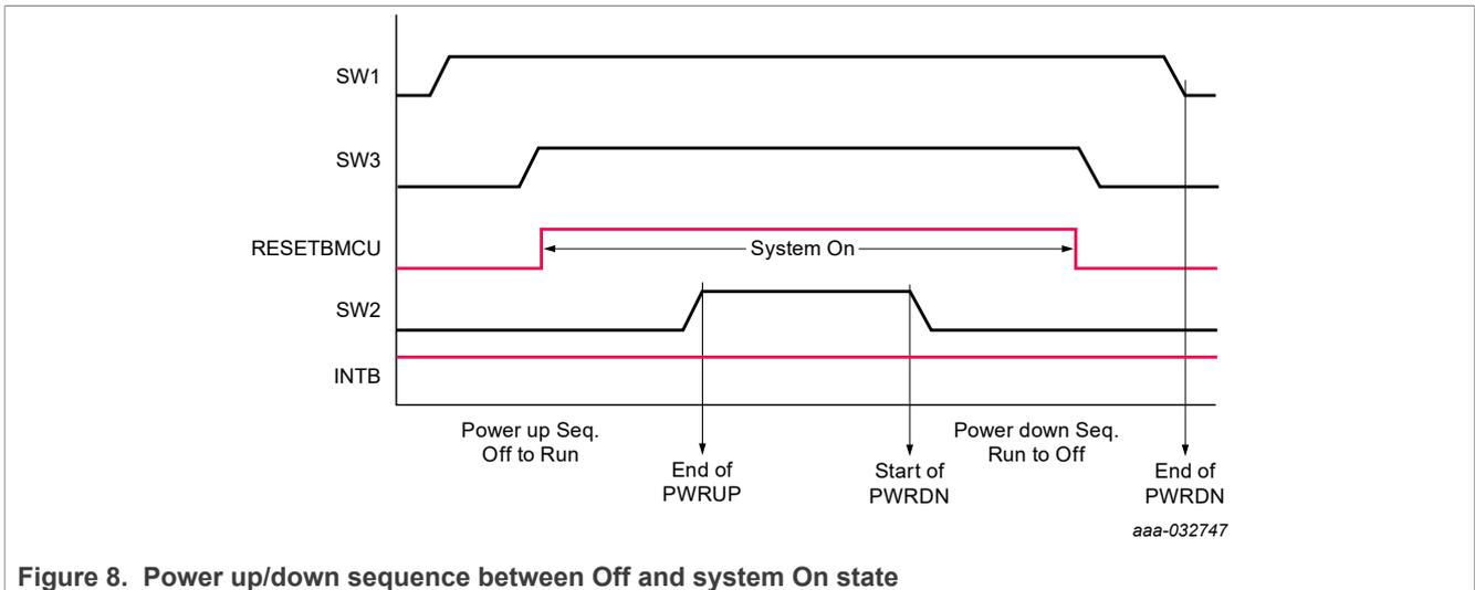
Figure 8. Power up/down sequence between Off and system On state
