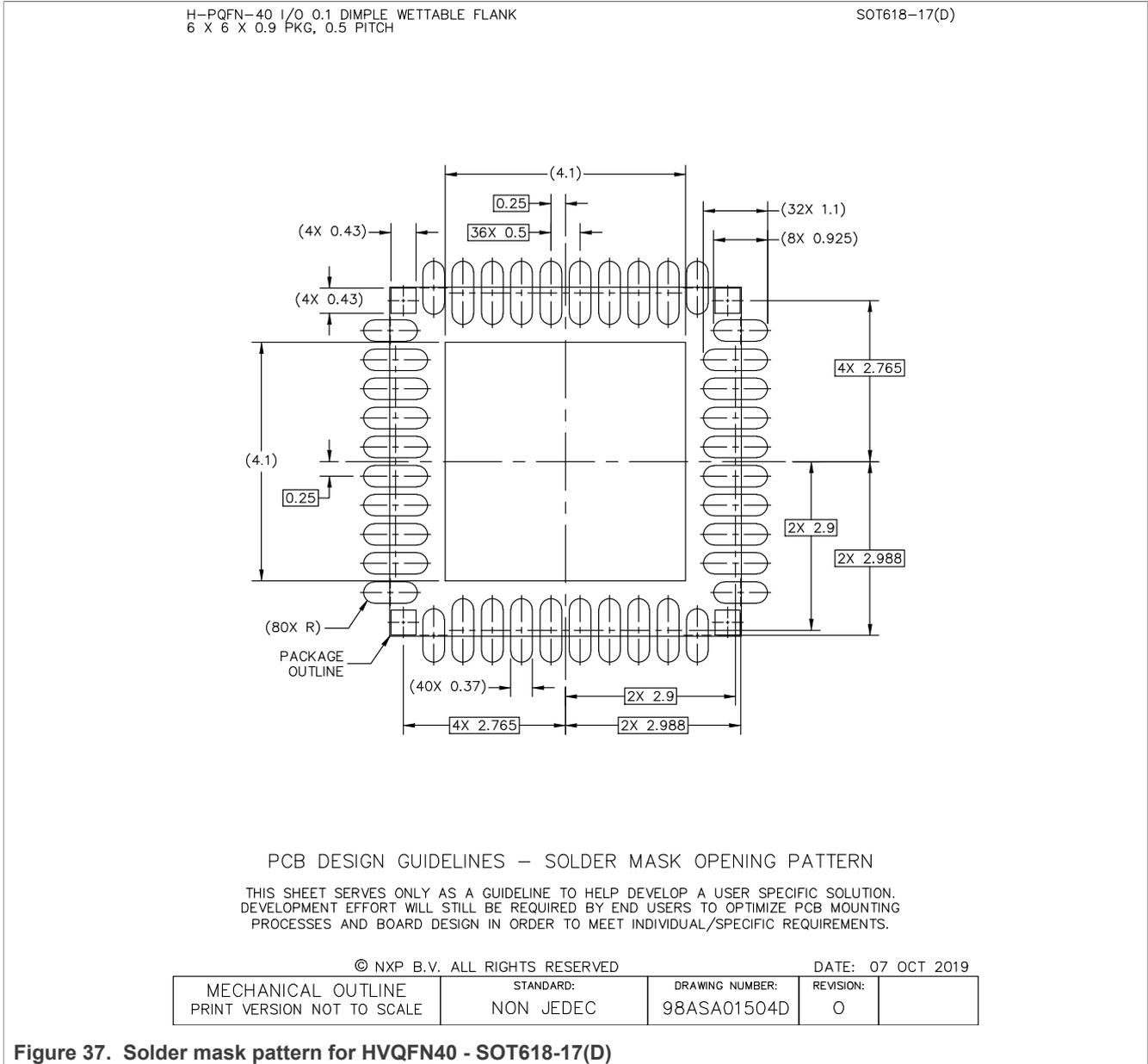
Figure 37. Solder mask pattern for HVQFN40 - SOT618-17(D)
