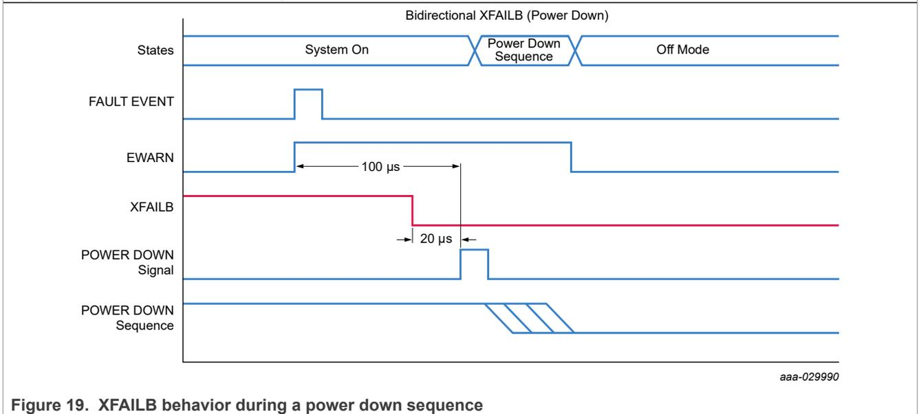
Figure 19. XFAILB behavior during a power down sequence
