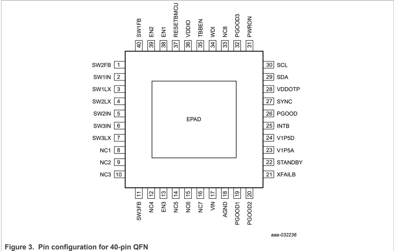
Figure 3. Pin configuration for 40-pin QFN
