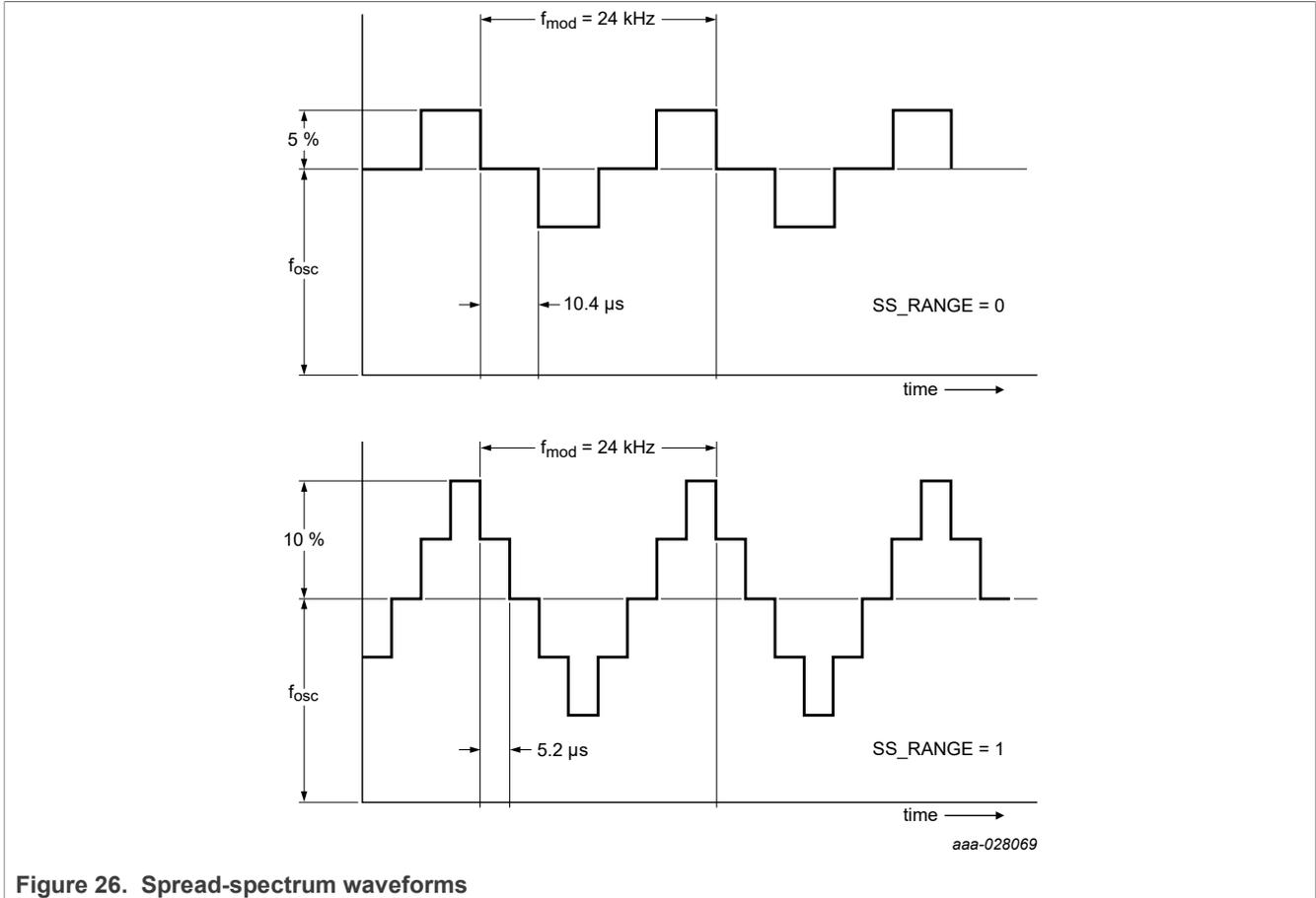
Figure 26. Spread-spectrum waveforms
