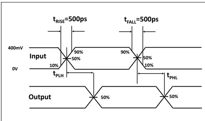
**Fig 5. Skew Test**
