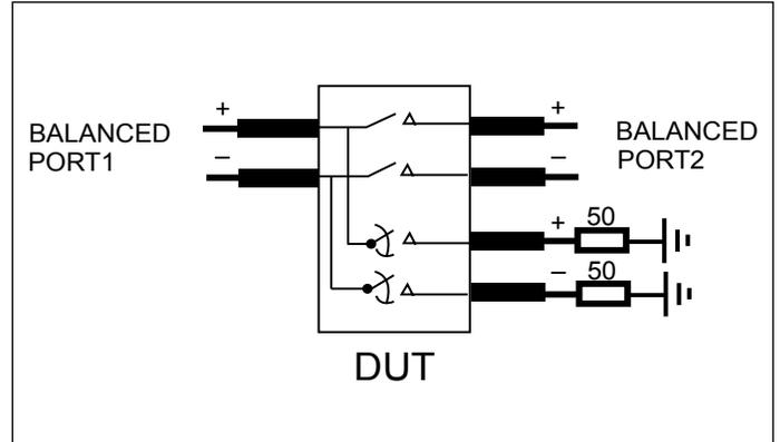
**Fig 2. Off-isolation Setup**
