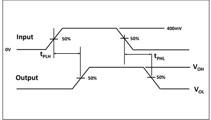
**Fig 4. Propagation Delay**
