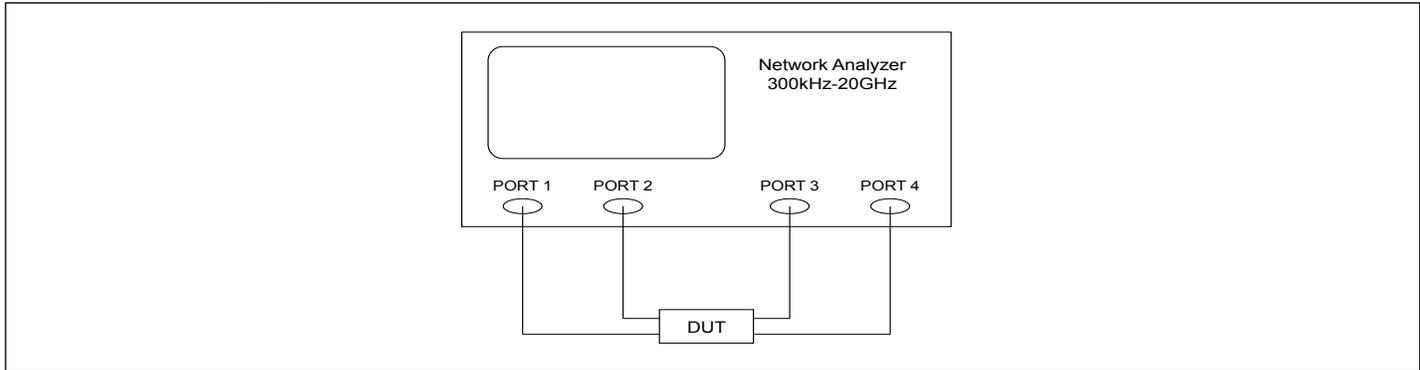
**Test Circuit for Electrical Characteristics<sup>(1-4)</sup>**
