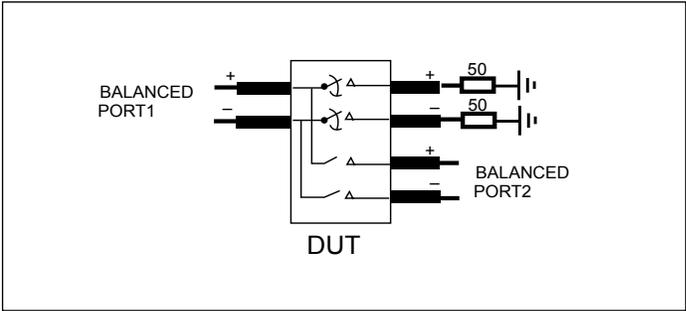
**Fig 2. Off-Isolation Setup**
