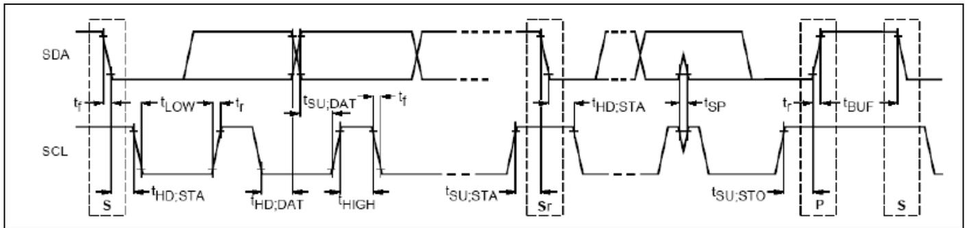
**Figure 1. Definition of Timing for Full-Speed Mode Devices on the I<sup>2</sup>C Bus**
