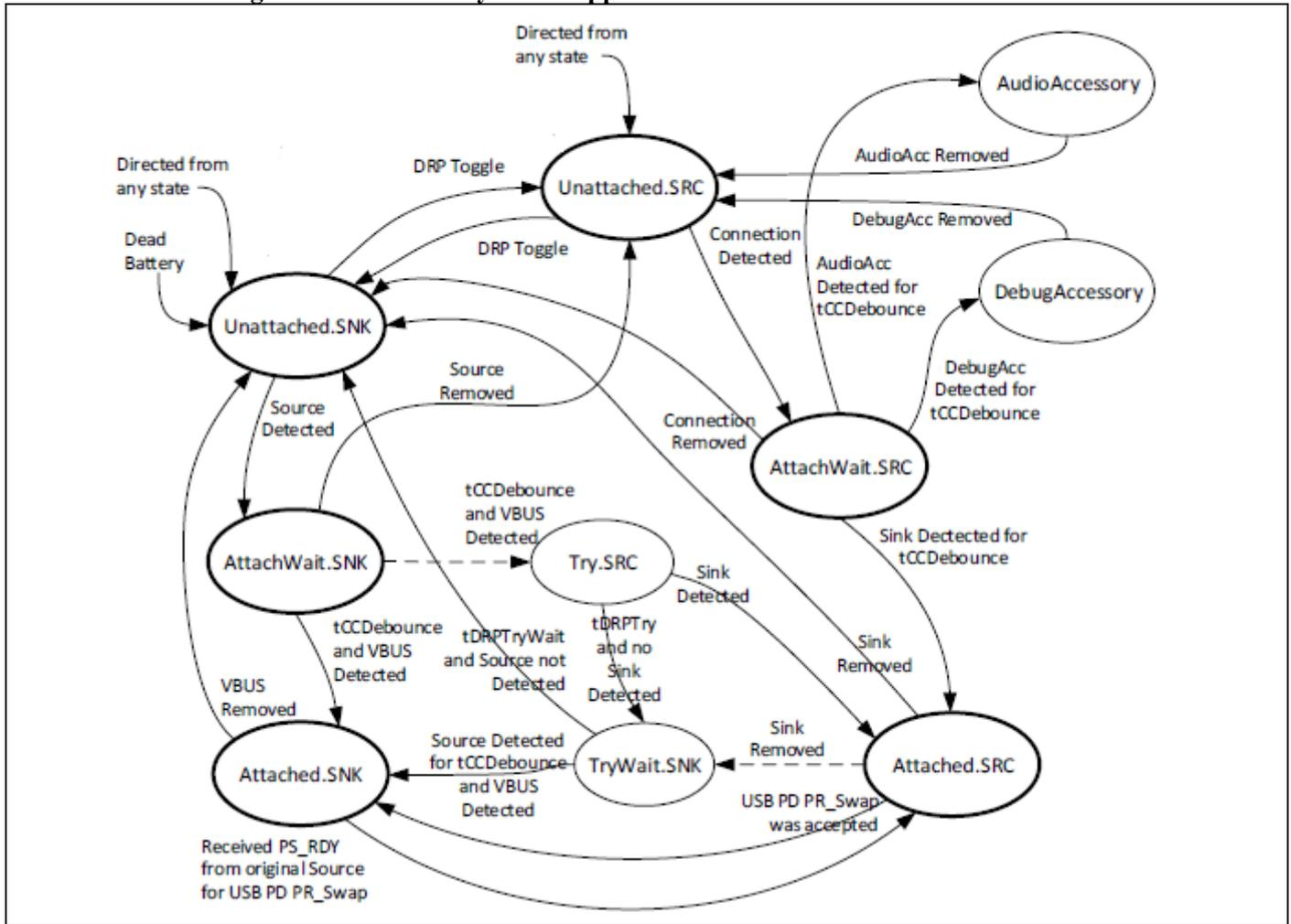
**Connection State Diagram: DRP with Try.SNK Supported**
