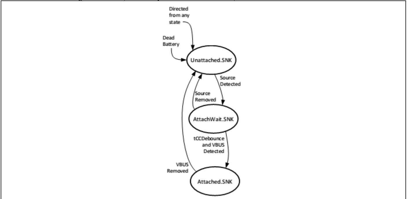
**Connection State Diagram: SNK (Accessory Detection is enable)**
