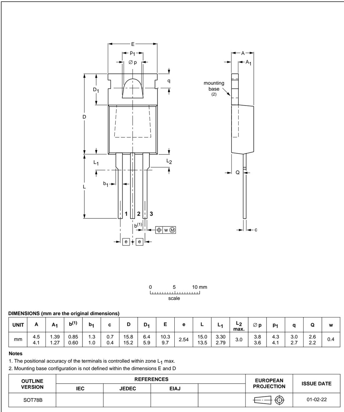
Fig.2. SOT78B (TO220AB) package<sup>1</sup>, pin 2 connected to mounting base.
