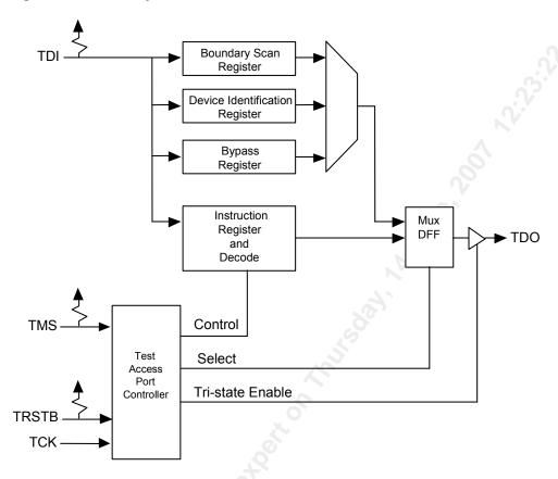
Figure 30 Boundary Scan Architecture
