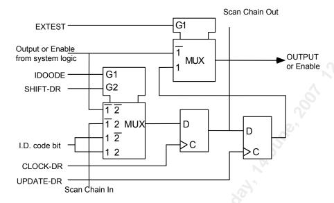
Figure 13 Bi-directional Cell (IO\_CELL)
