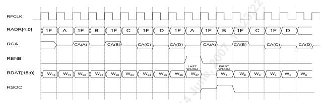
Figure 42 Receive UTOPIA Level 2 System Interface Timing(MPHY)
