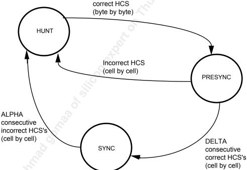
The values of ALPHA and DELTA determine the robustness of the delineation process. ALPHA determines the robustness against false misalignments due to bit errors. DELTA determines the robustness against false delineation in the synchronization process. ALPHA is chosen to be 7 and DELTA is chosen to be 6. These values result in an average time to delineation of 32  $\mu$ s for the STS-3c/STM-1 rate.
