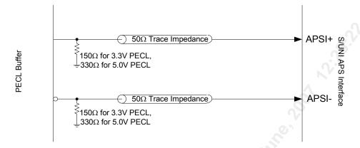
Figure 38 APS Interface between two PM5384 devices
