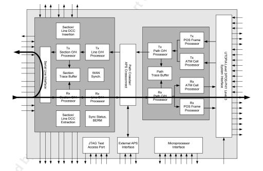
Figure 22 Line Loopback Mode
