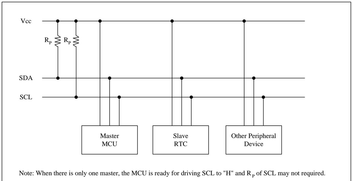
**Figure 1. System Configuration**
