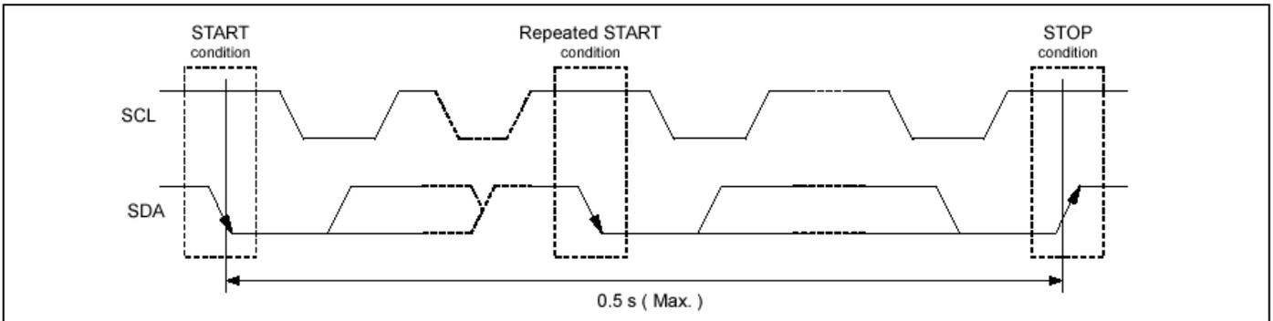
**Figure 2. Starting and Stopping on I<sup>2</sup>C Bus**
