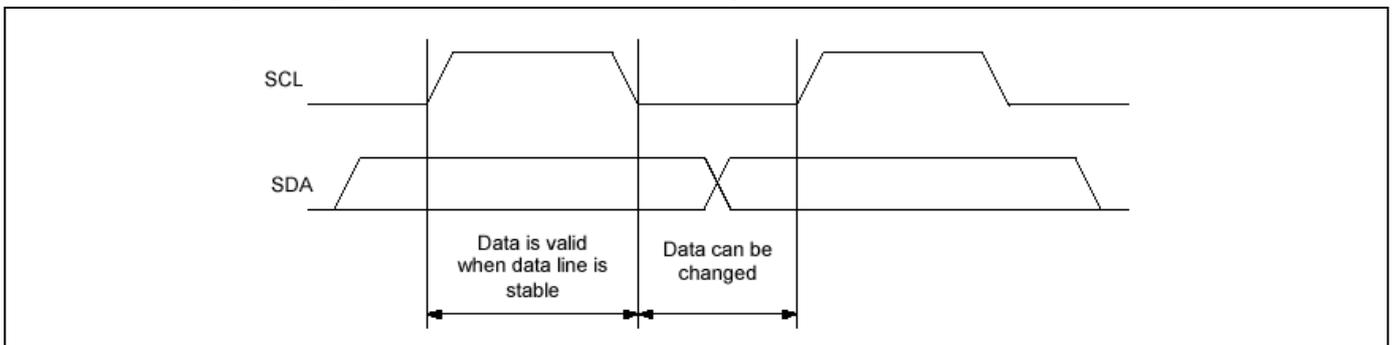
\*Note with caution that if the SDA data is changed while the SCL line is at high level, it is treated as a START, RESTART, or STOP condition.
