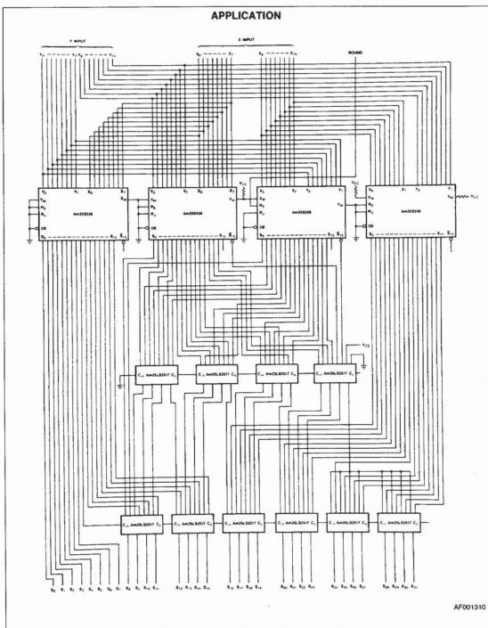
Figure 1. High-Speed 16 x 16 2's Complement Multiplication.
