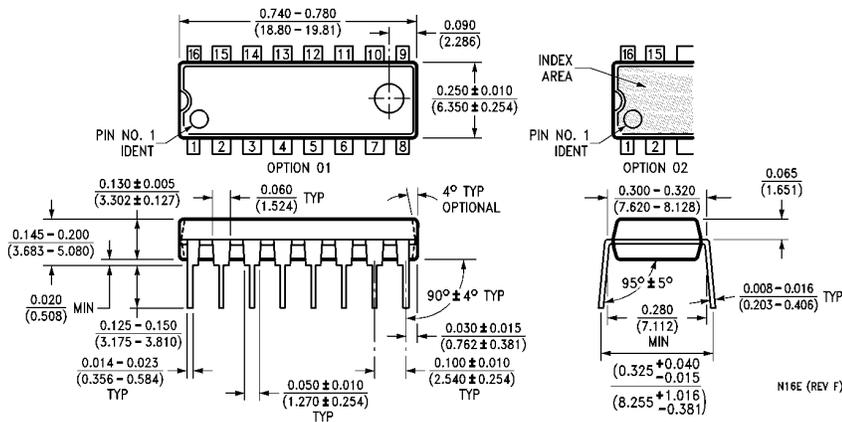
**16-Lead Molded Dual-In-Line Package (N)**
