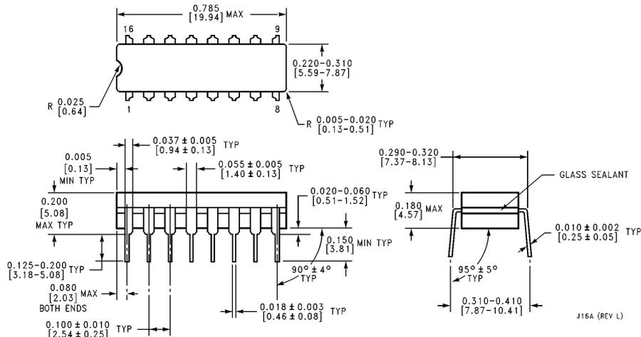
**16-Lead Ceramic Dual-In-Line Package (J)**
