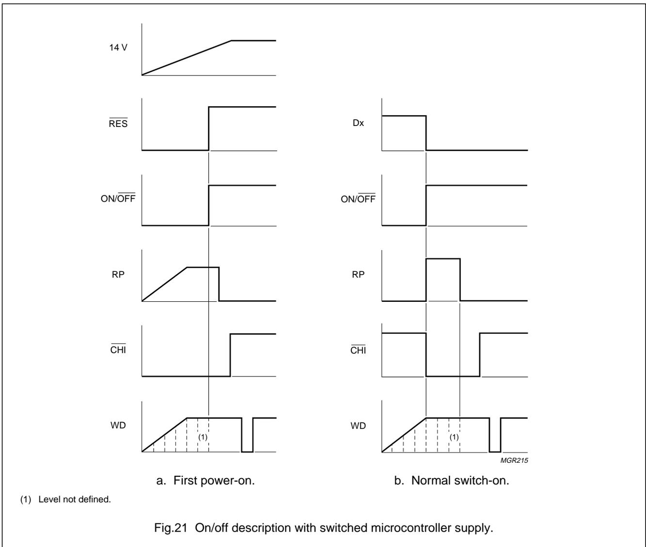
Fig.21 On/off description with switched microcontroller supply.
