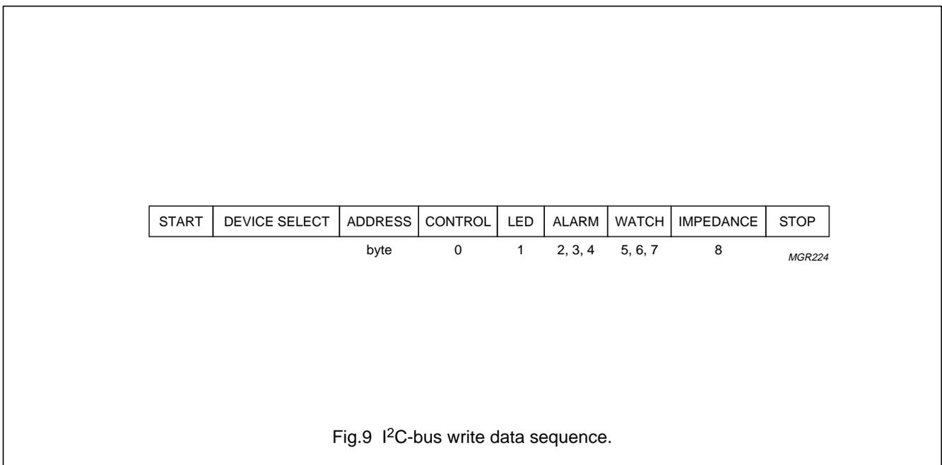
Fig.9 I<sup>2</sup>C-bus write data sequence.
