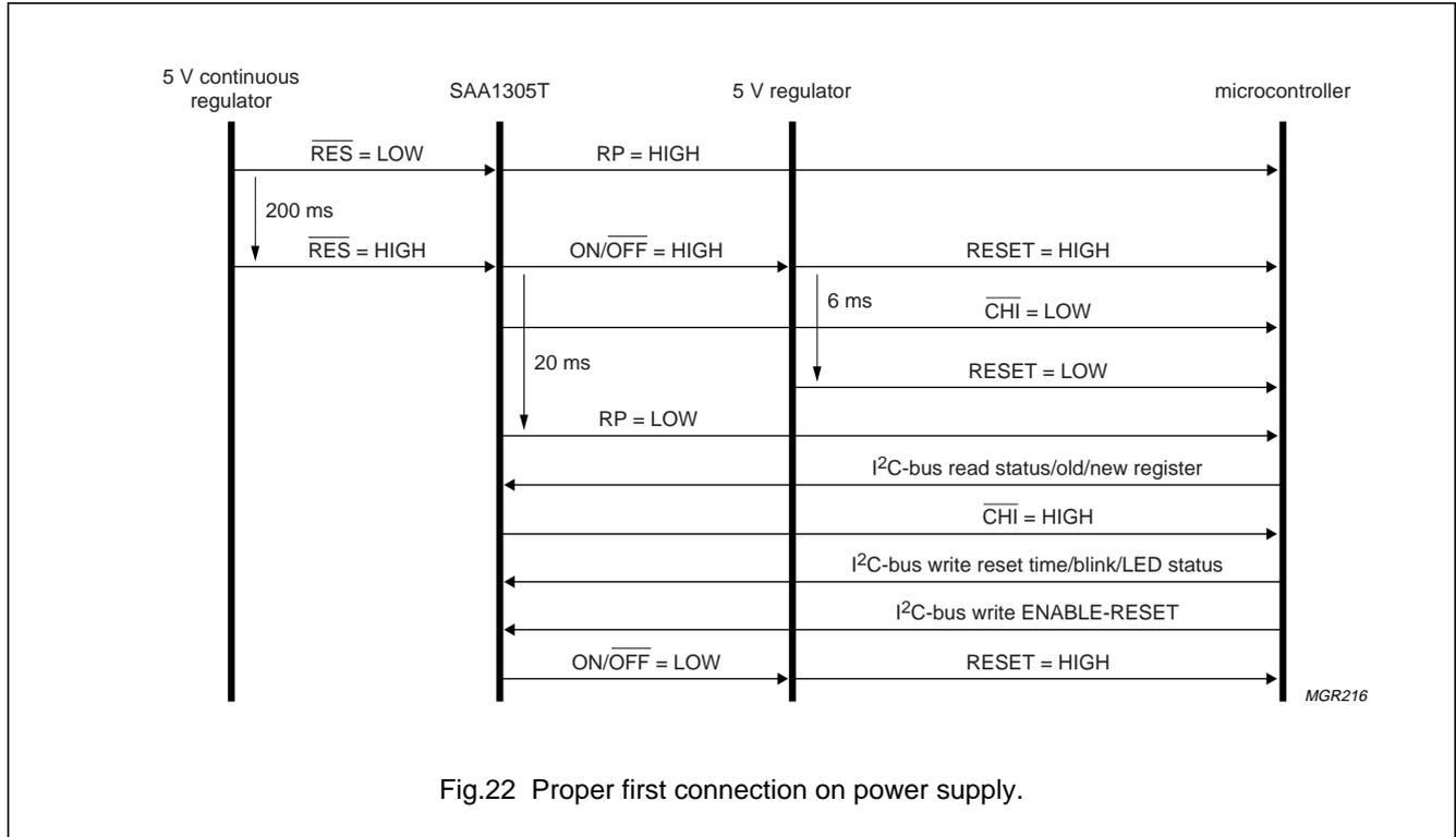
Fig.22 Proper first connection on power supply.
