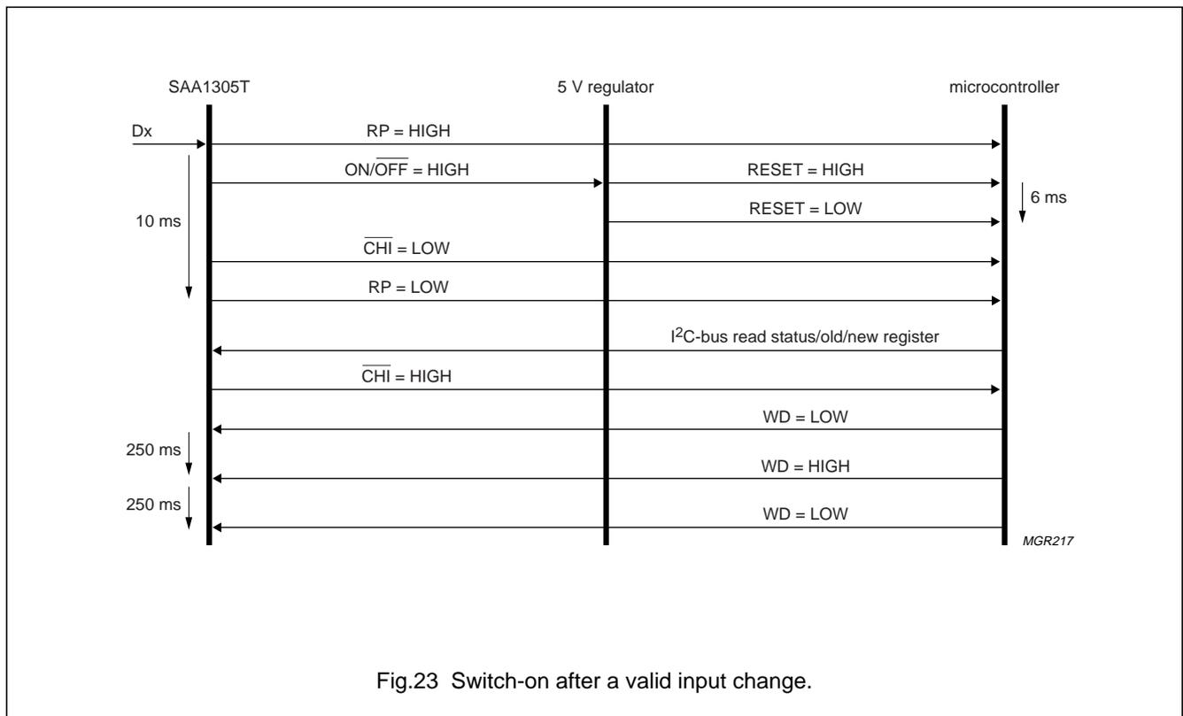
Fig.23 Switch-on after a valid input change.
