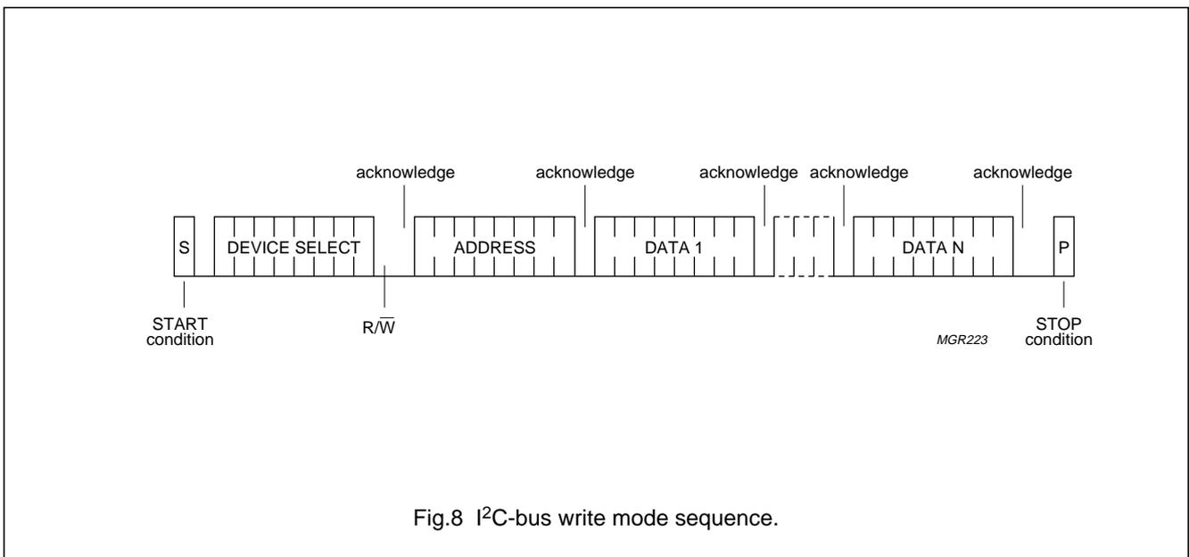
Fig.8 I<sup>2</sup>C-bus write mode sequence.
