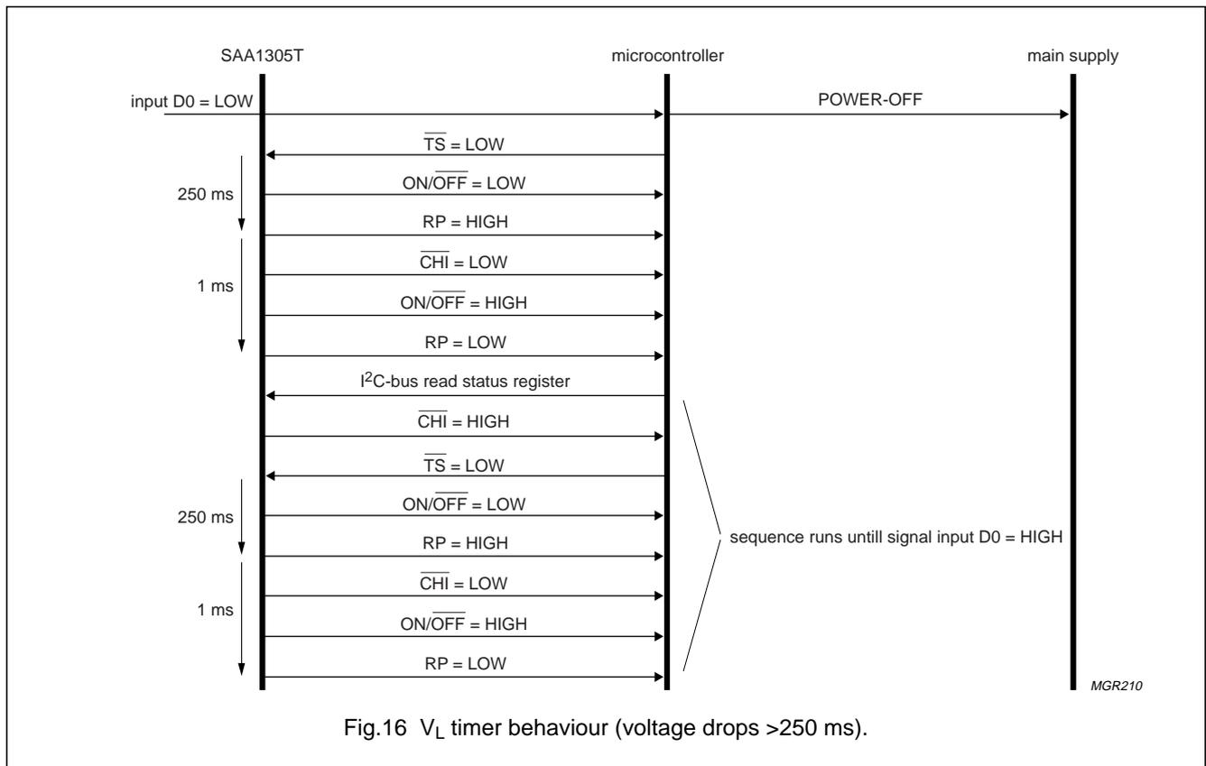
Fig.16  $V_L$  timer behaviour (voltage drops >250 ms).
