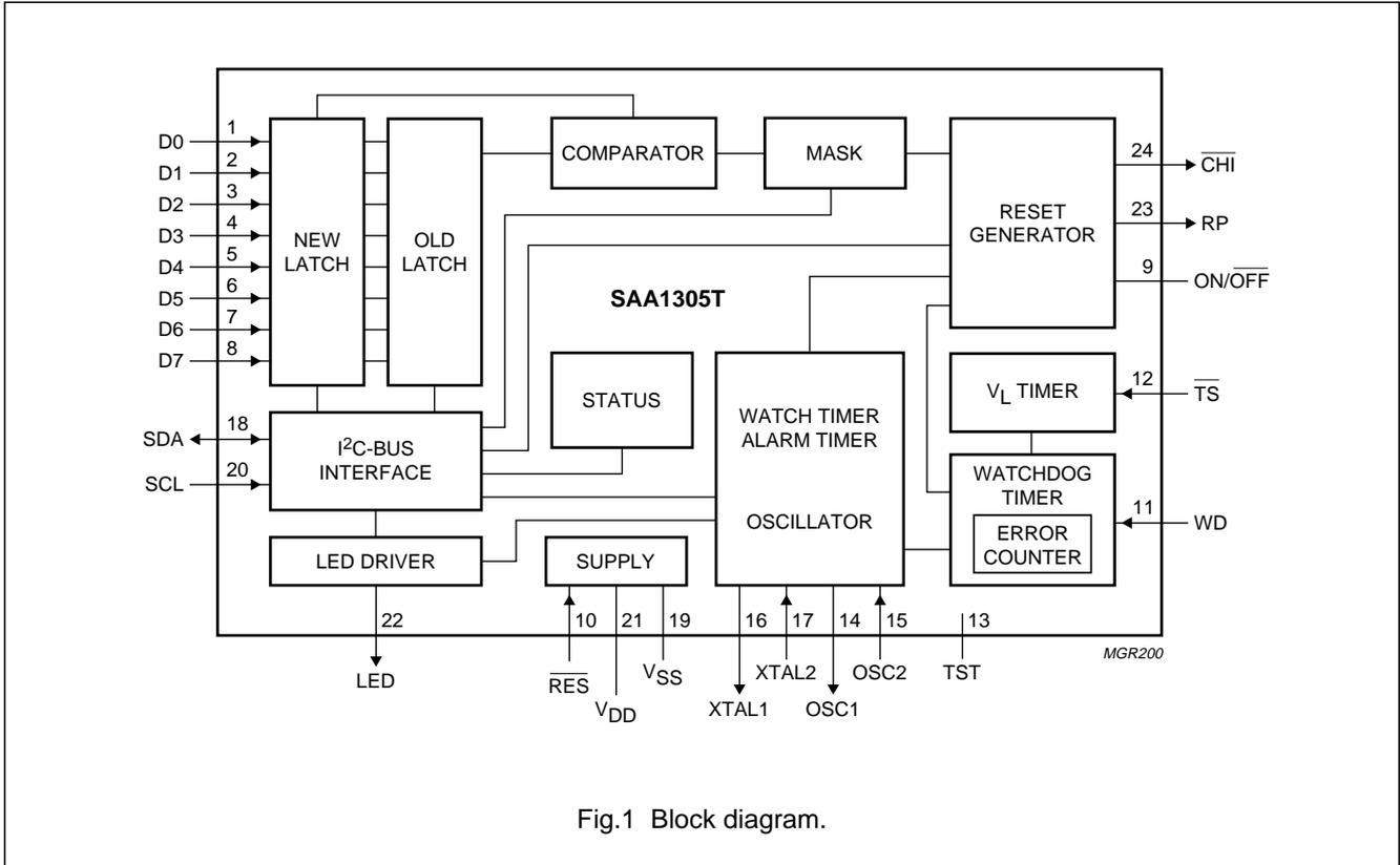
Fig.1 Block diagram.
