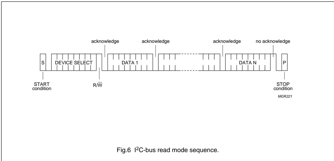
Fig.6 I<sup>2</sup>C-bus read mode sequence.
