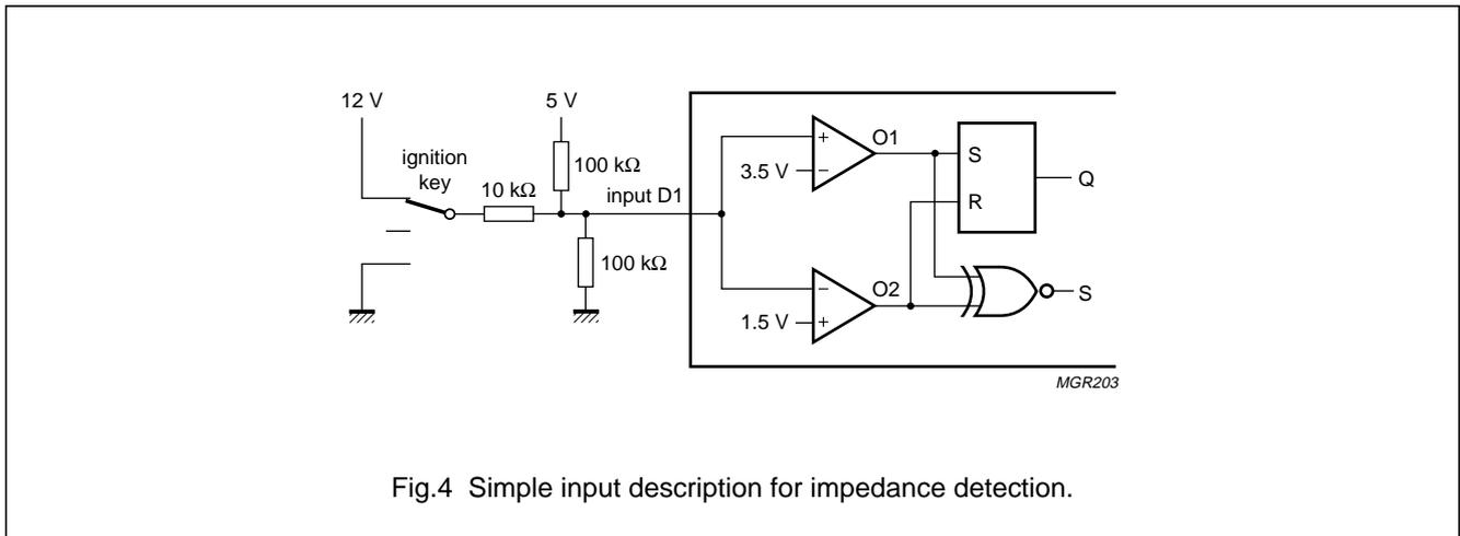
Fig.4 Simple input description for impedance detection.
