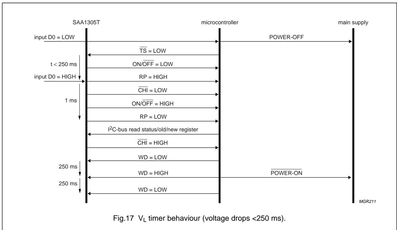
Fig.17  $V_L$  timer behaviour (voltage drops <250 ms).
