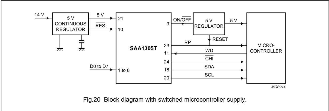
Fig.20 Block diagram with switched microcontroller supply.
