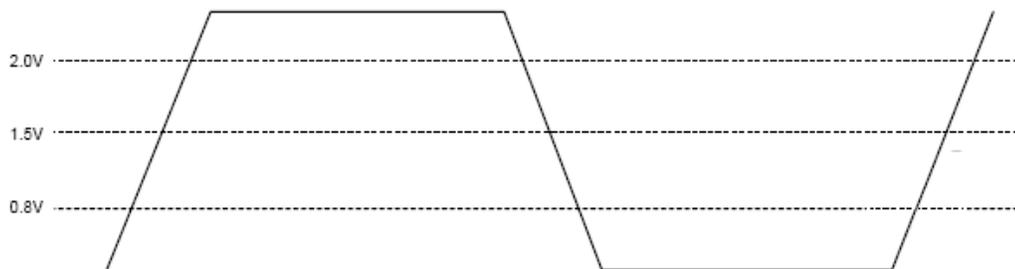
**Figure 4. Single-ended Output Signals (for AC Parameters Measurement)**
