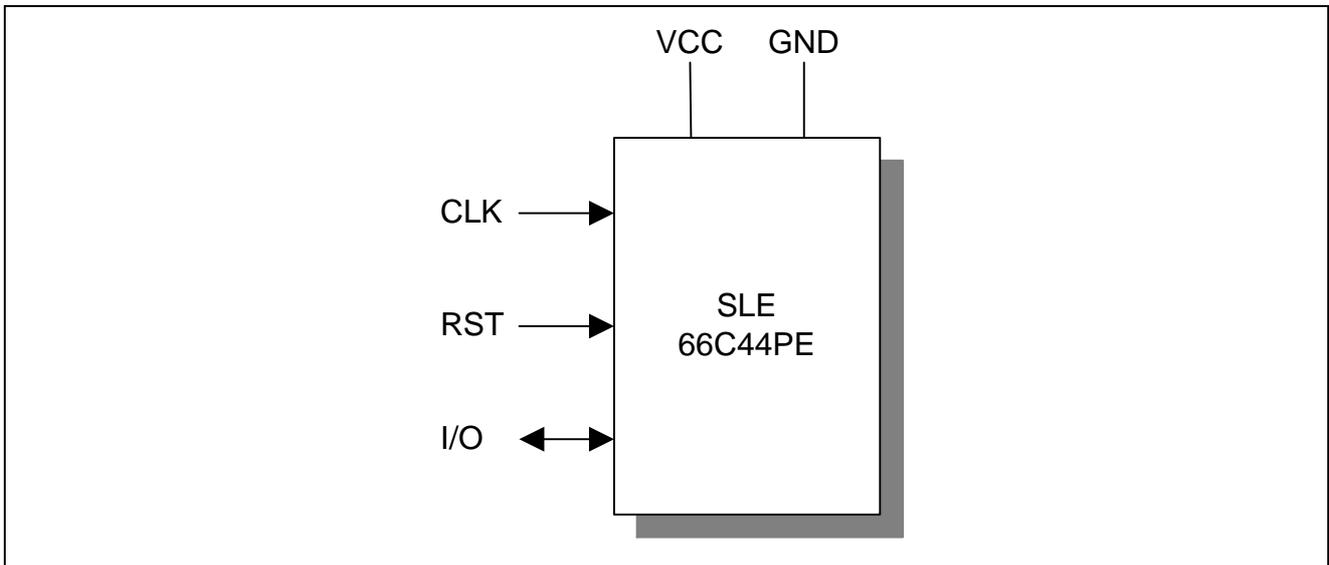
**Figure 1: Pin Configuration**
