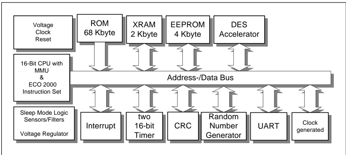
Figure 2: Block Diagram SLE 66C44PE
