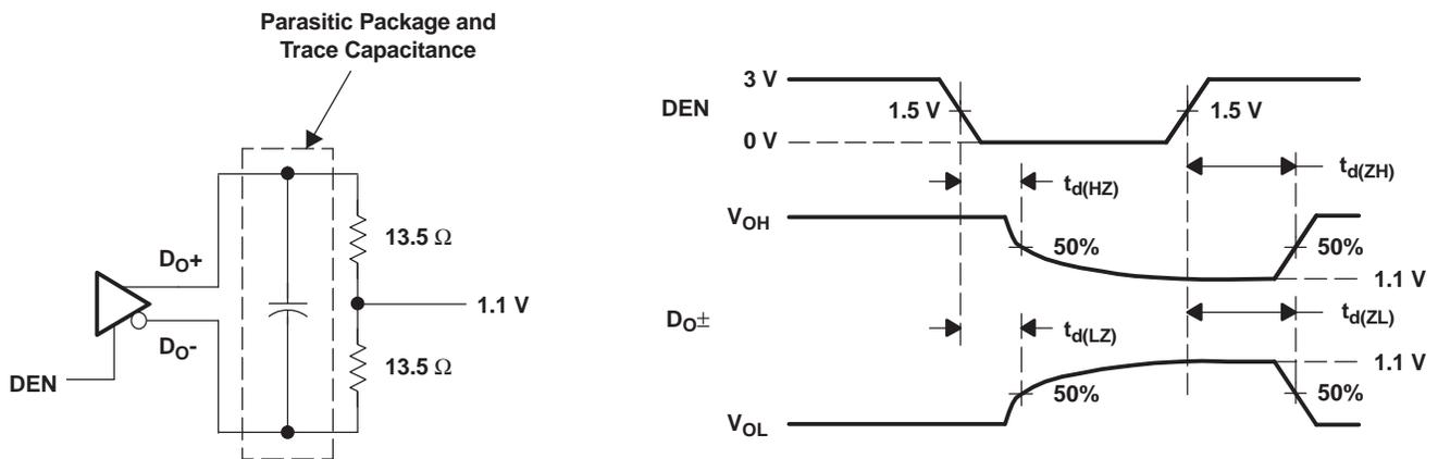
Figure 9. Serializer High-Impedance-State Test Circuit and Timing
