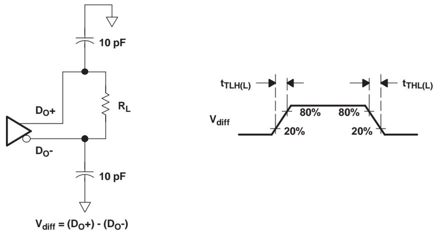
**Figure 5. Serializer LVDS Output Load and Transition Times**
