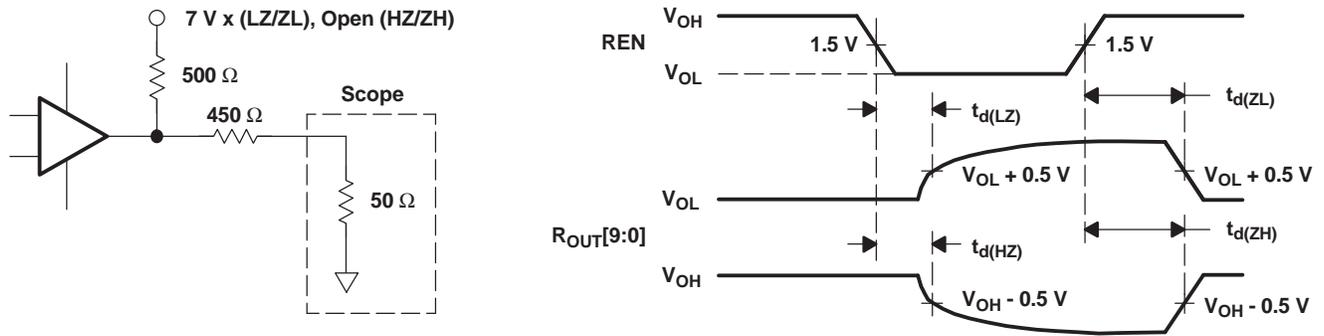
Figure 15. Deserializer High-Impedance-State Test Circuit and Timing
