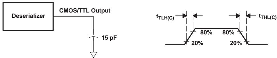
Figure 6. Deserializer CMOS/TTL Output Load and Transition Times
