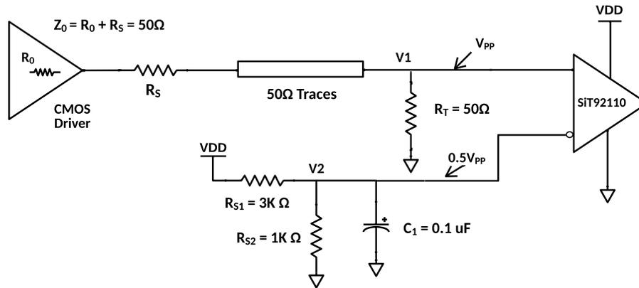
Figure 8 DC coupled LVCMOS input clock configuration – configuration 2
