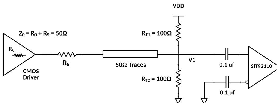
Figure 5 AC coupling LVCMOS clock to SiT92110
