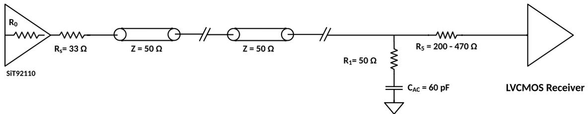
Figure 36 Different types of LVCMOS output clock termination with hot swap protection
