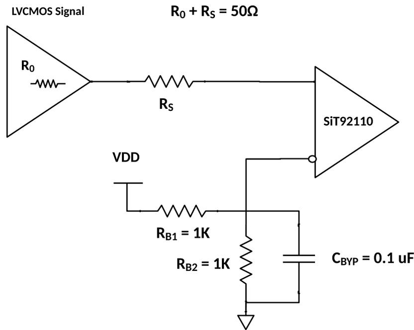
Figure 10: Direct coupling of LVCMOS clock to SiT92110
