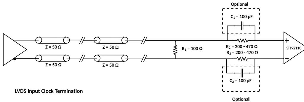
Figure 33 LVDS termination with hot swap protection
