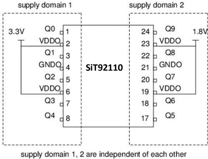
Figure 37: Example of multi supply operation of SiT92110
