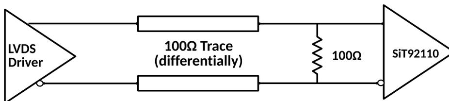
Figure 14 Termination scheme for DC coupled LVDS
