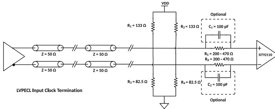
Figure 31 LVPECL termination with hot swap protection
