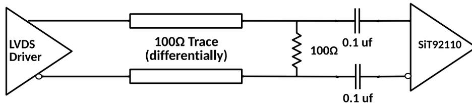
Figure 19 Termination scheme for AC coupled LVDS
